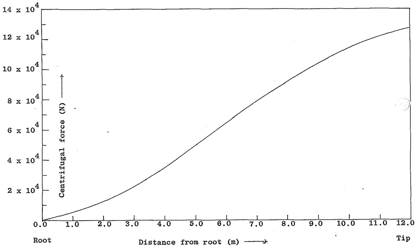
Fig.7. Distribution of centrifugal force along the 12m blade length at 60 RPM
