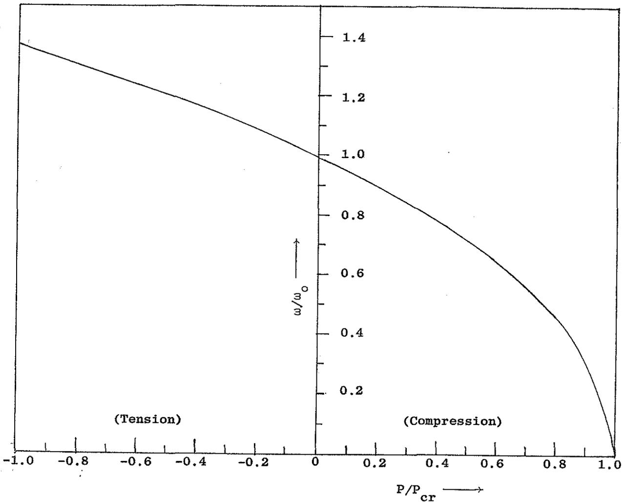
Fig.4. Effect of axial force (P) on the fundamental bending frequency ( $\omega$ ) of a uniform cantilever beam ( $\omega_0$  = frequency for the unloaded case;  $P_{cr}$  = Euler critical buckling load =  $\pi^2 EI/4L^2$ )
