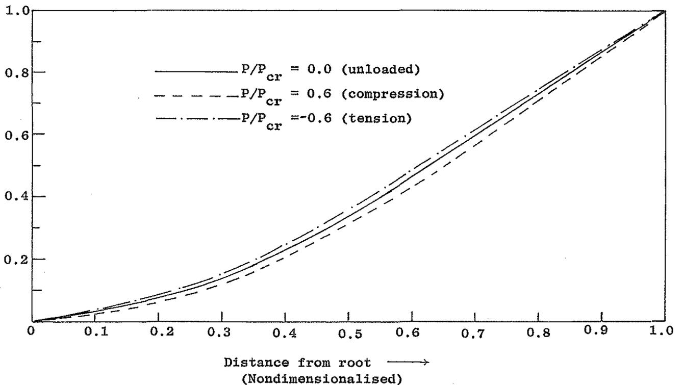
Fig.5. Effect of axial force on the fundamental bending mode of a cantilever beam ( $P_{cr}$  = Euler critical buckling load =  $\pi^2 EI/4L^2$ )
