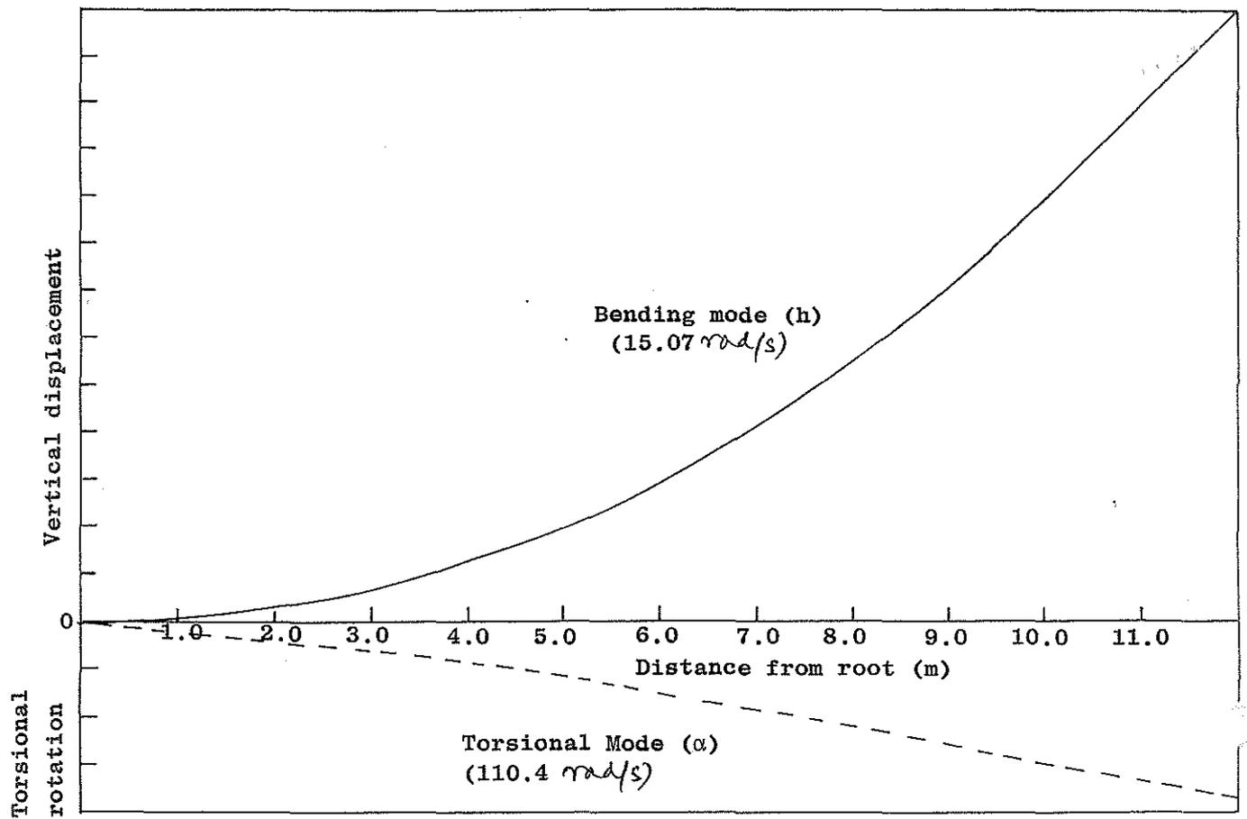
Fig.6. Fundamental bending and torsional (uncoupled) modes of 12m turbine blade.
