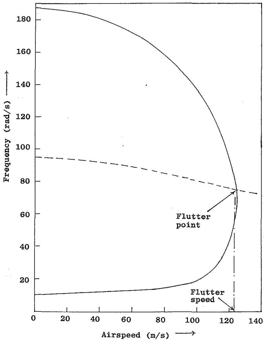
Fig. 2 Zeros of real and imaginary parts of flutter determinant, — roots of real part; ---- roots of imaginary part.
