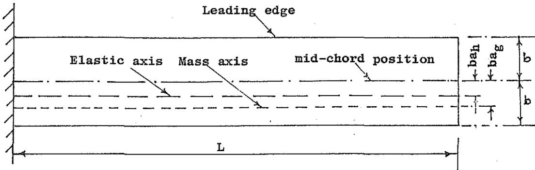
Fig.1 A uniform aerofoil blade with cantilever end condition
