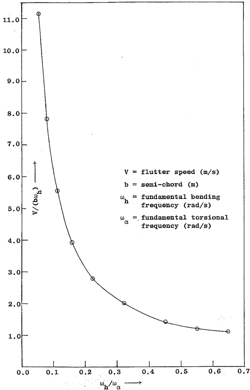
Fig.3. Flutter speed coefficient  $V/(b\omega_h)$  as function of frequency ratio  $\omega_h/\omega_\alpha$  of cantilever blade.
