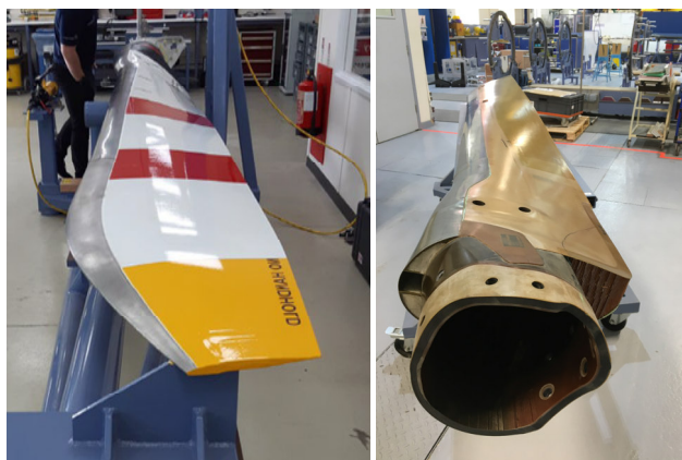
Figure 2 –New generation Enhanced Tiltrotor Blade (also known as the RGF blade)
