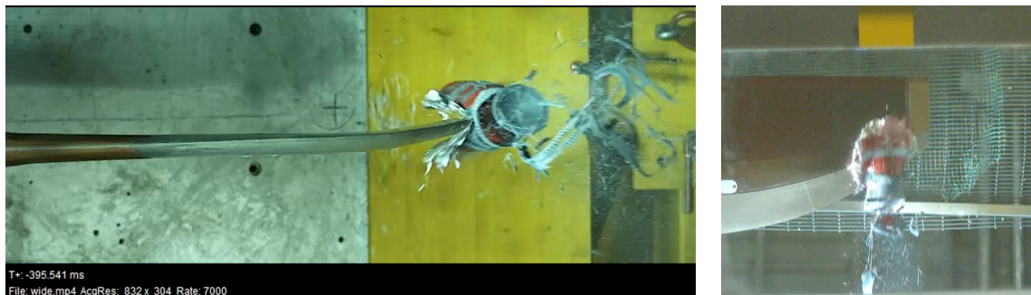
Figure 19 – Physical bird-strike tests were performed using gel-based surrogate bird projectiles (POLIMI test facility)
