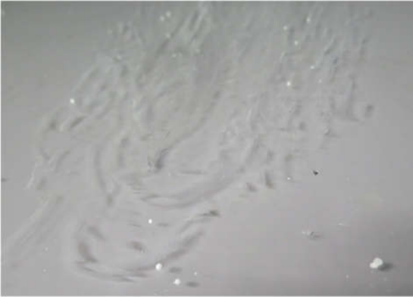
Figure 10 Surface scratches on windshield of canopy demonstrator at drone impact location
