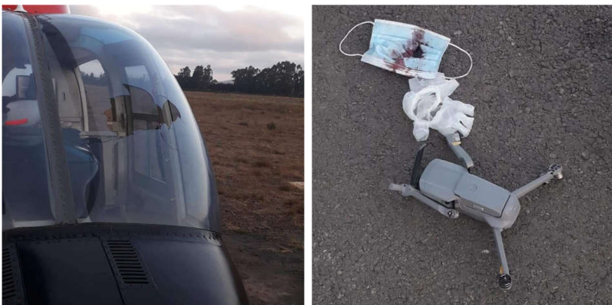
Figure 3 Midair collision in June 2020 on a Bell UH-57B with a cracked windshield and injuries to occupant [5]
