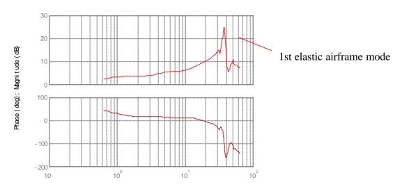
Figure 8: Helicopter transfer function in hover for the pilot seat - ECD
