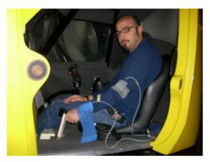
Figure 11: Experimental test set-up with acceleration sensors applied to the arm of the pilot
