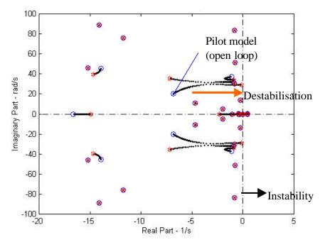
Figure 9: Closed loop system for hover - ECD
