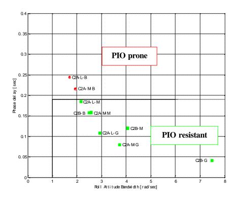
Figure 6: Bandwidth phase delay criterion for roll axis in hover conditions - ONERA
