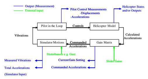
Figure 13: Test scheme for aeroelastic RPC
