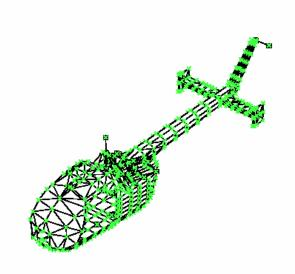
Figure 4: BO105 Finite Element Airframe Model
