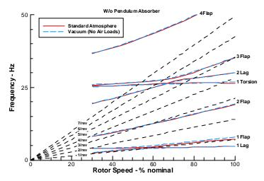
Figure 3: Fan diagram of BO105 aeroelastic rotor model
