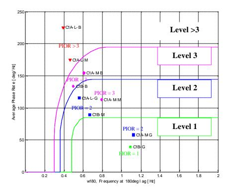
Figure 5: Average phase rate criterion for pitch axis in forward flight - ONERA
