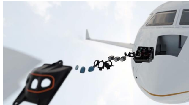
Fig. 4. “Exploded” view of a modern enhanced vision system showing the three independent multispectral channels that are fused into a single real time image for the cockpit crew. Credits: Collins Aerospace.
