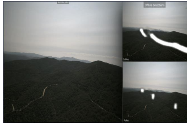
Fig. 10. Development view of the AI-based system showing the raw output of a neural network over visual frames from onboard cameras, highlighting objects (wires, masts) potentially recognised as hazards. Video can be seen here: Ref. 38. Credits: Daedalean
