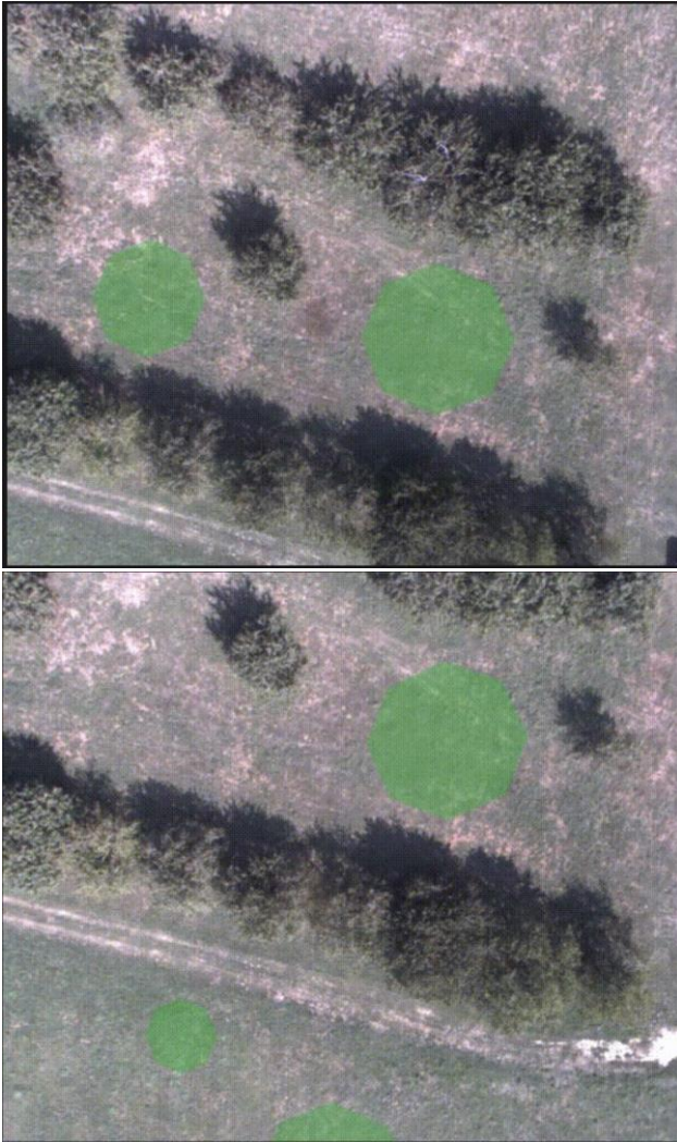
Fig. 11-12: Example of a visual vertical landing system detecting a suitable landing zone in unprepared terrain, video can be seen here: Ref. 39. Credits: Daedalean
