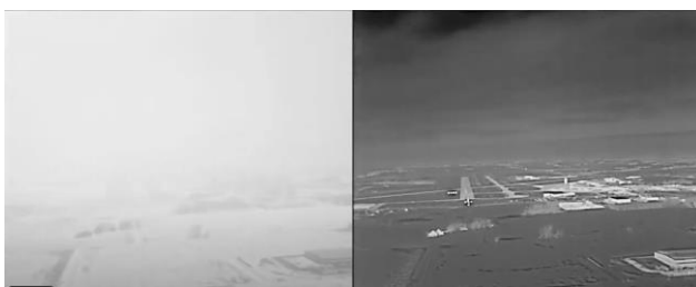
Fig. 3. Example of low-visibility “equivalent visual” operation from an enhanced vision system such as those proposed in this paper. Left: out-the-window (unaided) view. Right: same view, through an enhanced-vision system (video can be seen in Ref. 28). Credits: Collins Aerospace.
