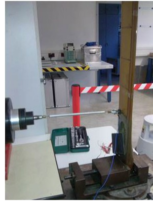
Figure 2. Blade frequency measurement setup at DLR laboratory.
