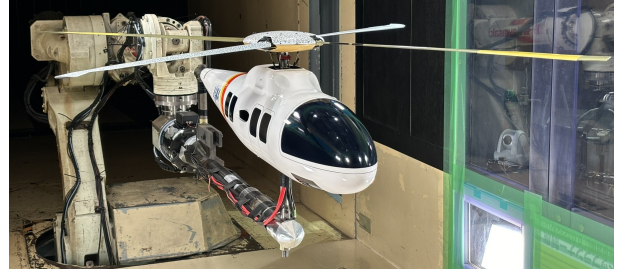
Figure 1: Helicopter test model in the JAXA LWT2
