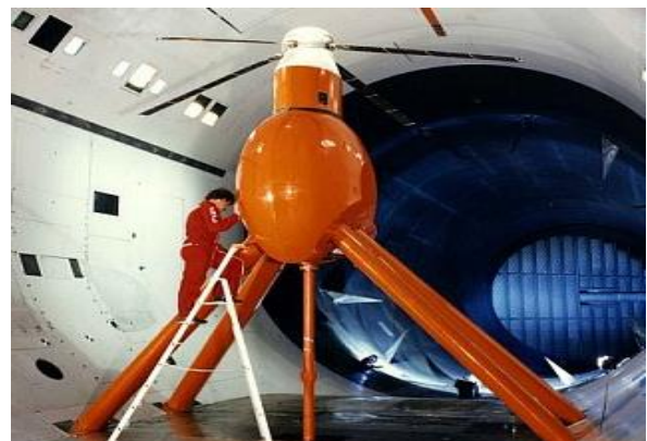
Figure 1: 7AD isolated rotor in ONERA S1 wind tunnel.
