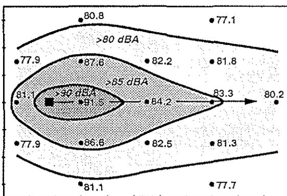
Figure 22: Comparison between measurement and prediction of the noise ground contour for 10° take-off with the modified model
