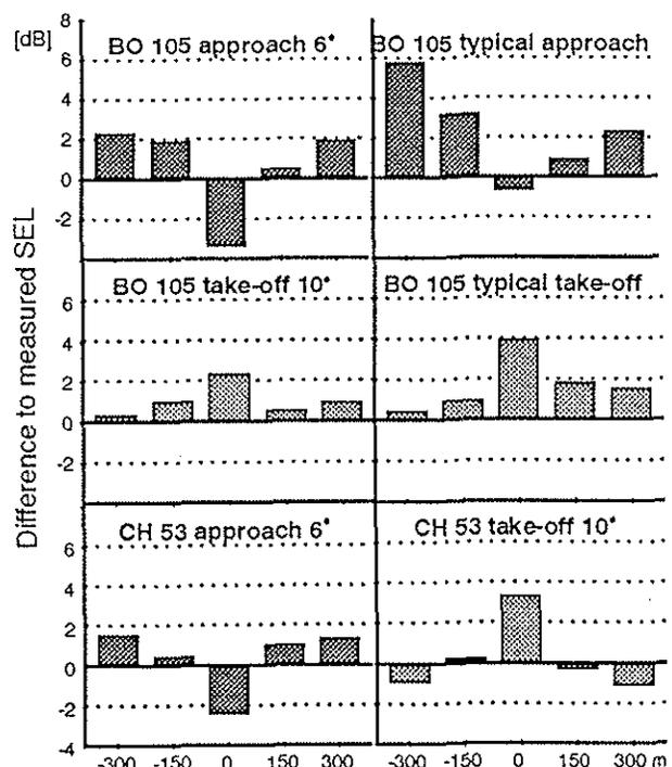
Figure 21: Differences of predicted SEL-equivalent values of the modified model with measured SEL-values
