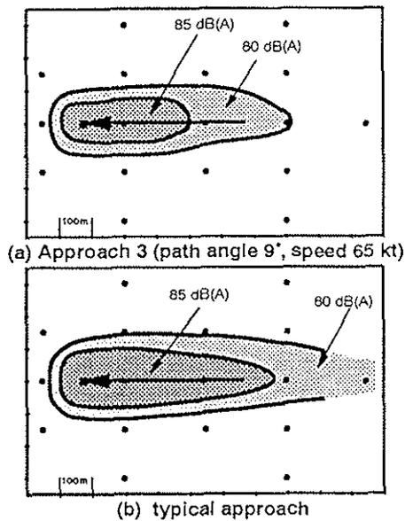
Figure 7: BO 105 approaches:  $L_{Amax}$ -ground contours
