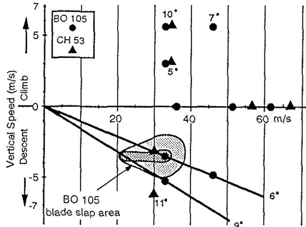
Figure 5: Test matrix for the BO 105 and the CH 53
