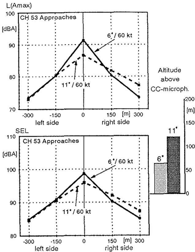
Figure 10: CH 53:  $L_{A_{max}}$ - and SEL-levels for approach conditions (microphone line 625 m ahead of the landing point)
