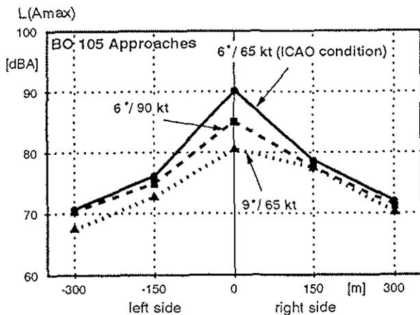
Figure 8: BO 105:  $L_{Amax}$ -levels for the approach conditions (microphone line 625 m ahead of the landing point)
