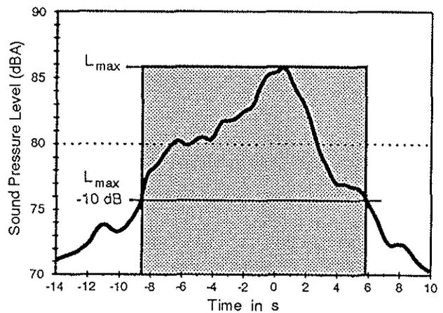
Figure 16: Flyover noise level based on the maximum noise level and duration of the noise event
