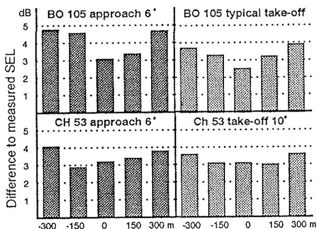
Figure 18: Deviations of SEL-equivalent values with measured SEL values
