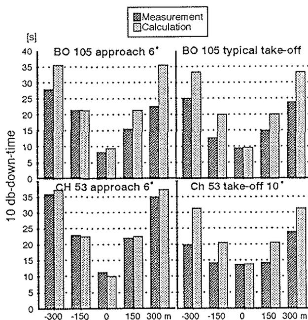
Figure 19: Comparison of measured 10-dB-down-times with prediction formulation
