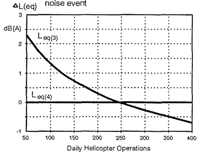
Figure 17: Differences of  $L_{eq(q=3)}$  and  $L_{eq(q=4)}$  versus number of flights
