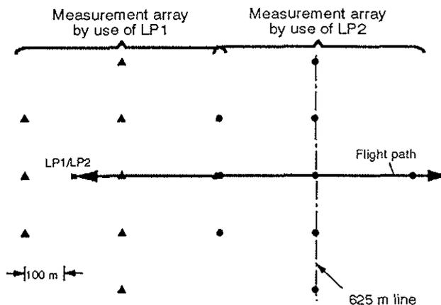
Figure 2: Enlarged measurement array by two landing points LP1 and LP2
