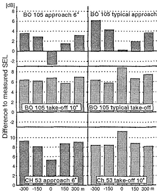
Figure 20: Differences of predicted SEL-equivalent values with measured SEL-values (calculated in accordance to the Air Traffic Control Act)
