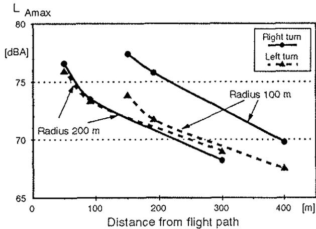
Figure 15:  $L_{Amax}$ -levels for BO 105 turn flight conditions
