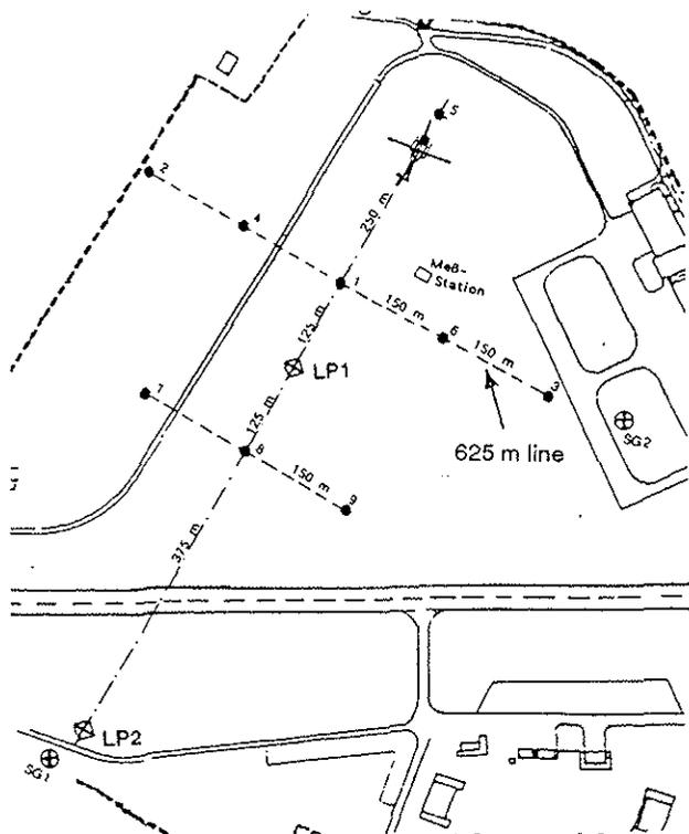
Figure 1: Measurement array: SG1 and SG2 are the positions of the flight path tracking system, LP1 and LP2 are the hover locations for the take-off and approach tests
