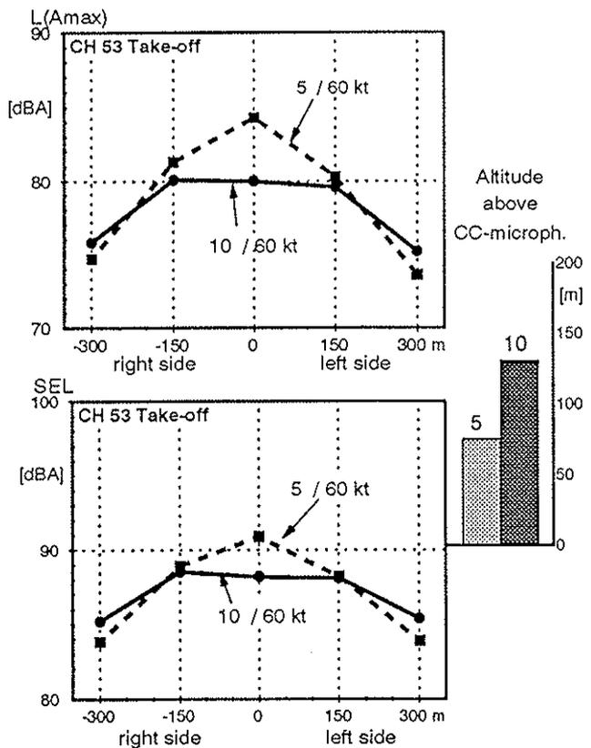
Figure 14: CH 53:  $L_{Amax}$ - and SEL-levels for take-off conditions (microphone line 625 m ahead of the landing point)
