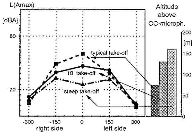
Figure 12: BO 105:  $L_{Amax}$ -levels for take-off procedures (microphone line 625 m away from the landing point)
