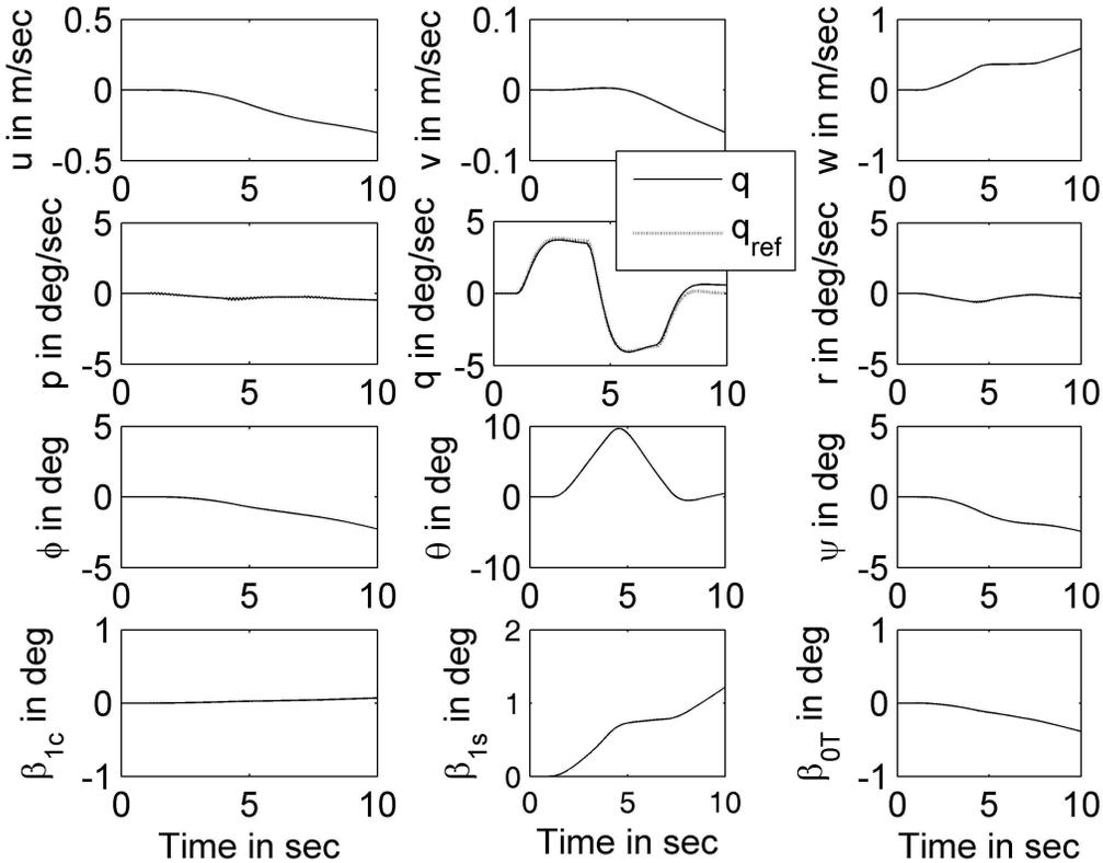
Fig. 7. Helicopter Response for Obstacle Clearance Maneuver.
