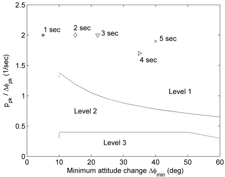
Fig. 9. Roll attitude quickness criterion at nominal flight condition.
