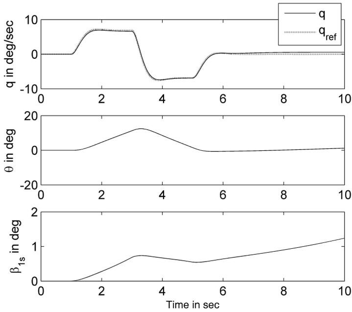
Fig. 3. Helicopter response and control surface deflection for pitch attitude command signal.
