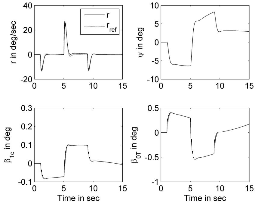
Fig.5. Helicopter response and control surface deflection for yaw rate command signal
