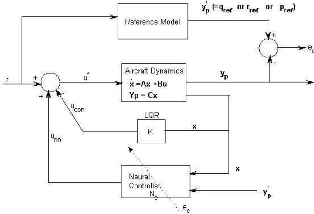
Fig. 1. Block diagram of feedback error learning neural control (FENC) Scheme
