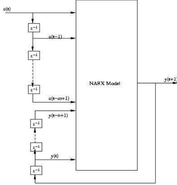
Fig.2 Nonlinear Auto Regressive eXogeneous Input Network Architecture.
