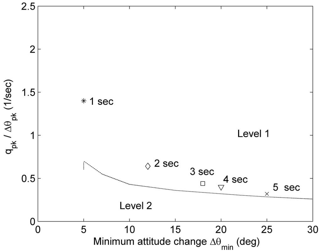
Fig. 8. Pitch attitude quickness criterion at nominal flight condition.
