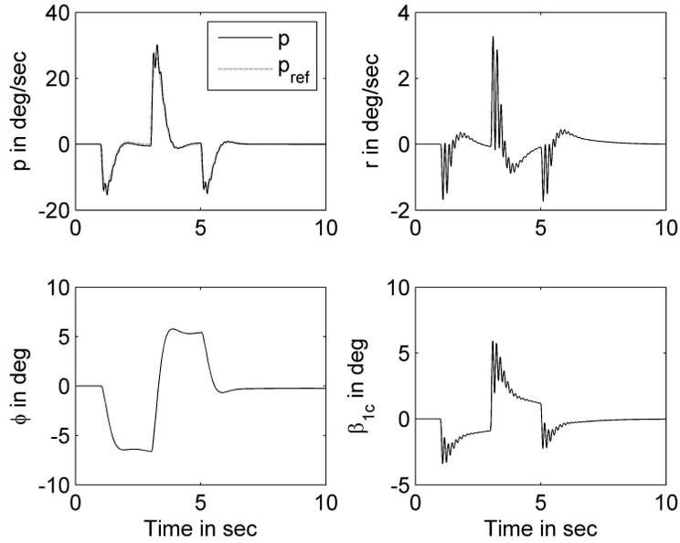
Fig. 4. Helicopter response and control surface deflection for roll rate command signal.
