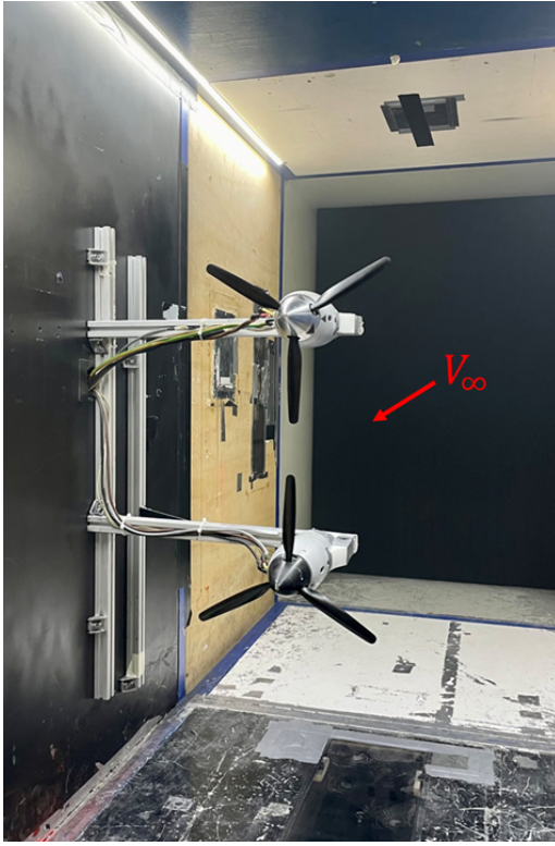
Figure 1. Layout of the VRS side-by-side propellers experimental setup at S. De Ponte wind tunnel of Politecnico di Milano.
