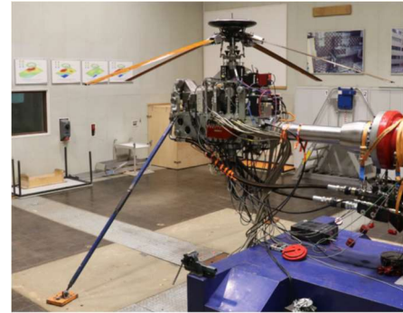
Figure 3: Test setups for rotating natural frequencies of STAR blades (Courtesy of DLR).
