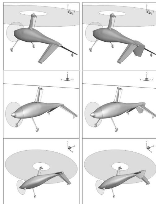
Figure 7. Comparison geometry autogyro I-28 B (left) with the geometry of a modified version I-28 B mod.1 (right)
