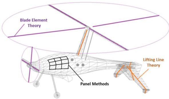
Figure 11. Different methods for simulating the dynamics of the autogyro flight
