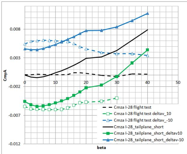
Figure 9. Influence of rudder deflection ( $\delta v = \pm 10^\circ$ ) difference between equipped with tailplate and flight test configuration [9]
