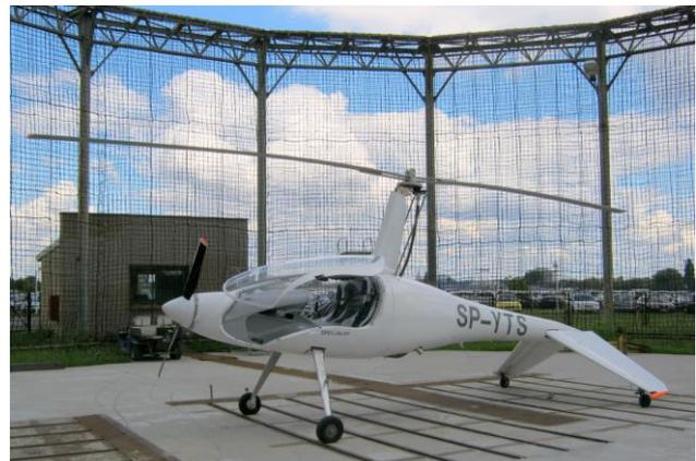
Figure 1. Autogyro I-28B in test rotors stand at the Institute of Aviation
