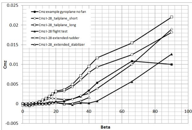
Figure 8. Yaw moment function of sideslip angle for analyzed configurations [9]
