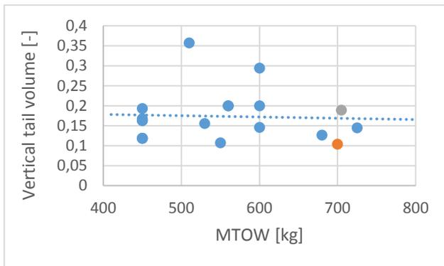
Figure 6. Vertical tail volume in function of MTOW
