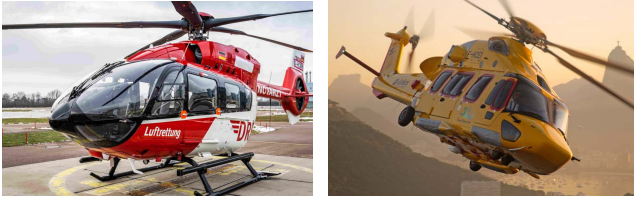
Figure 1: Picture of the Airbus H145 helicopter with skid landing gear (Ref. 3) and the Airbus H175 helicopter with retractable wheeled landing gear (Ref. 4)
