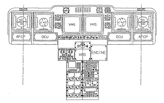
b - The VMS functions are designed to provide the crew members with every parameter necessary to control the engines as well as the various vehicle systems and, should a system failure be detected, by providing guidance for corrective actions.
