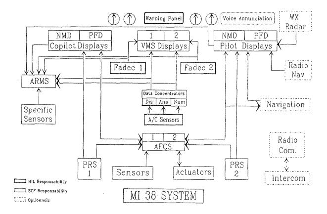
MI38's system architecture is based on ARINC 429 data links with the exception of specific equipment e.g. weather radar for which special standards are defined.
