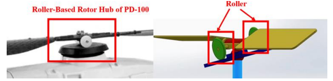
Figure 2: Roller-based rotor hub of PD-100
