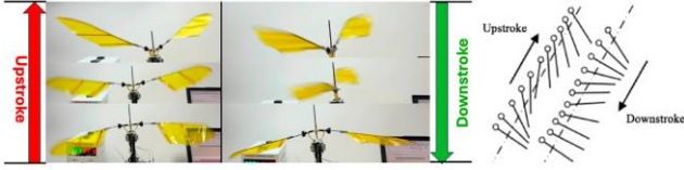
Figure 8: Hybrid FWR wing motion during one flapping cycle
