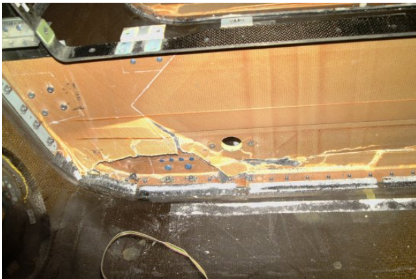
Pic.38: Damages in sub-floor frames energy absorbing zone
