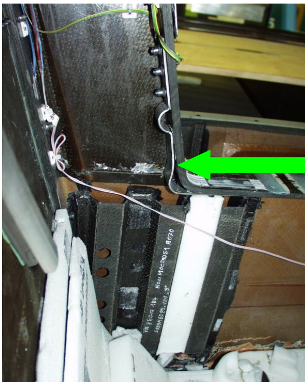
Pic.39: Crack and crack stopper in lower frame corner
