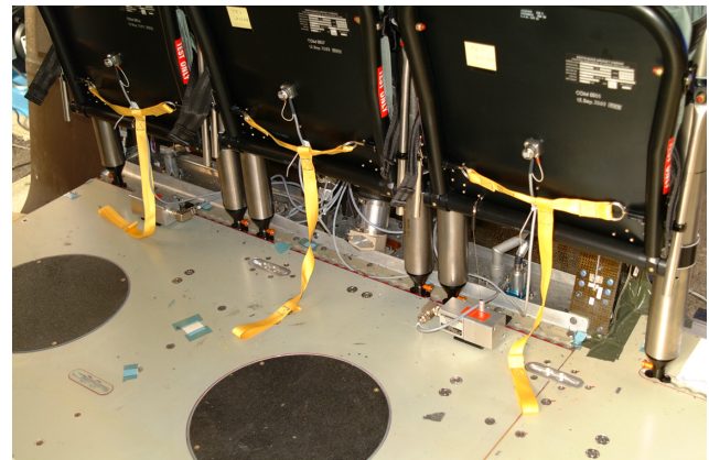
Pic.32: No damage was found in the interface between the seat poles and the floor panel
