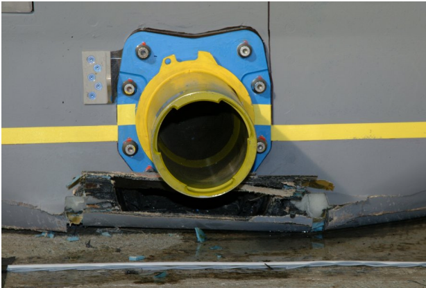
Pic.33: Pintle Axle after test: available stroke below was sufficient
