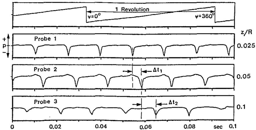
Figure 14. Probe signals of the blade vortices
