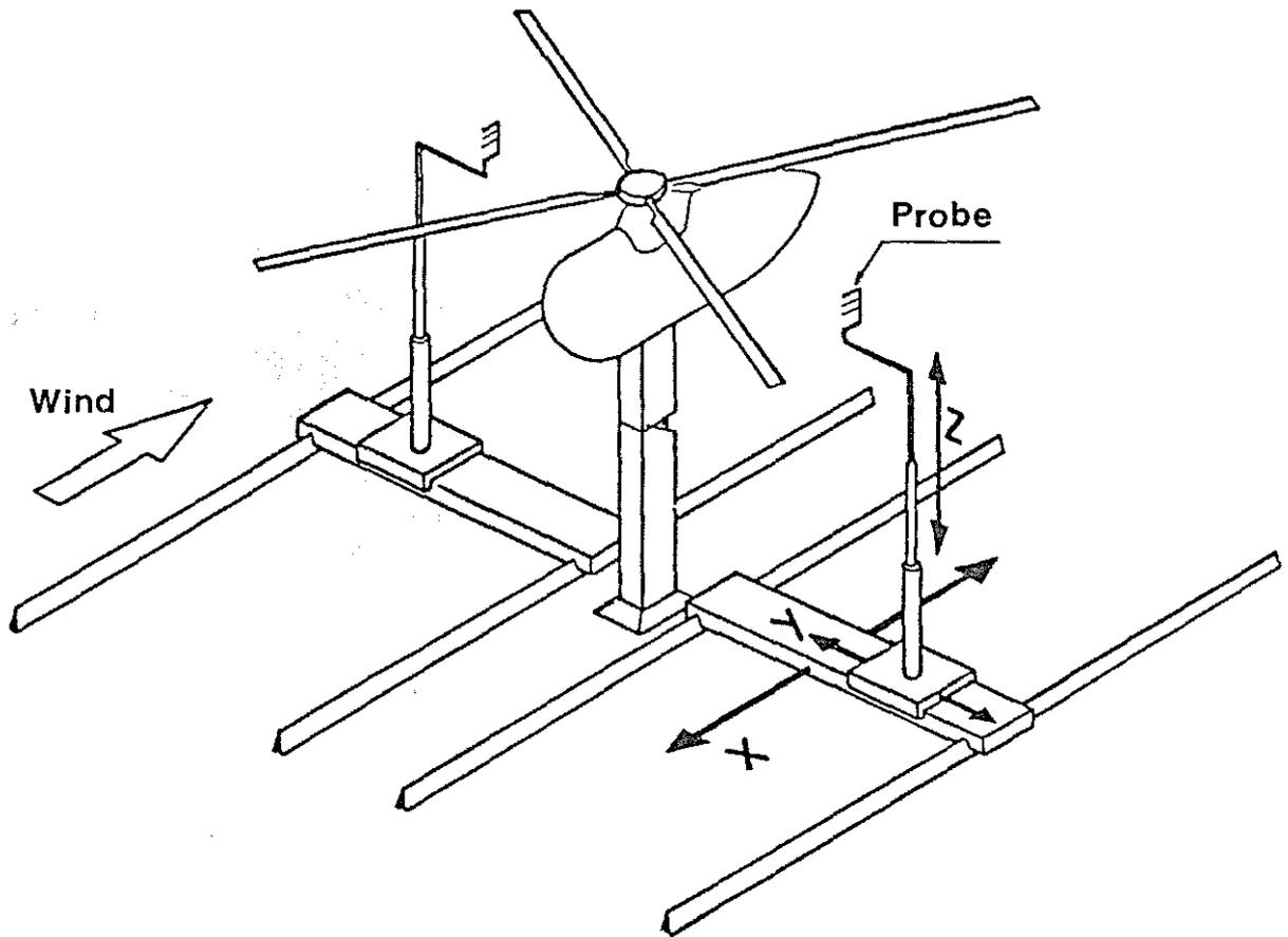
Figure 1. DFVLR-Rotor-Teststand with the downwash measuring equipment
