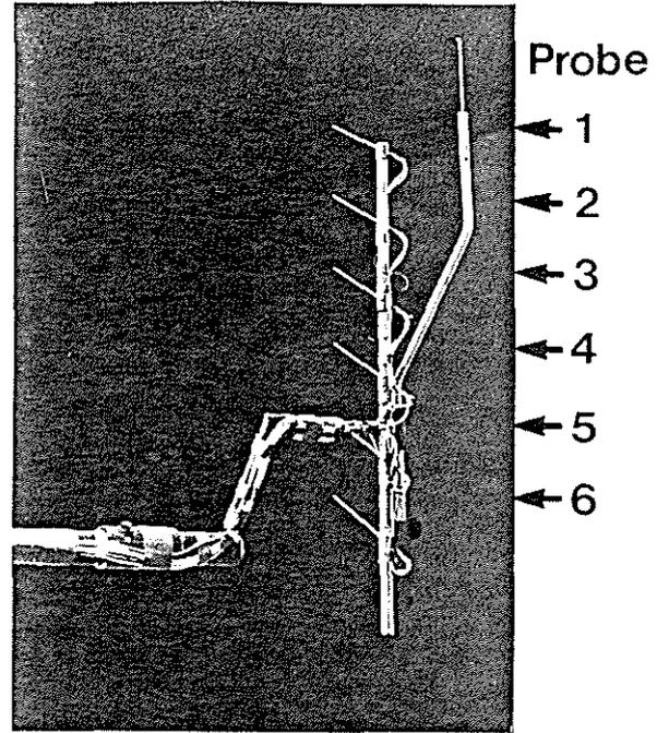
Figure 4. Dynamik pressure probe rake
