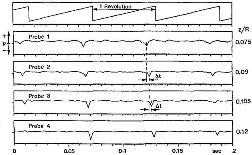
Figure 13. Probe signals of the trim-tab vortex
