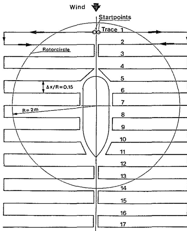
Figure 5. Traces of the probes below the rotor
