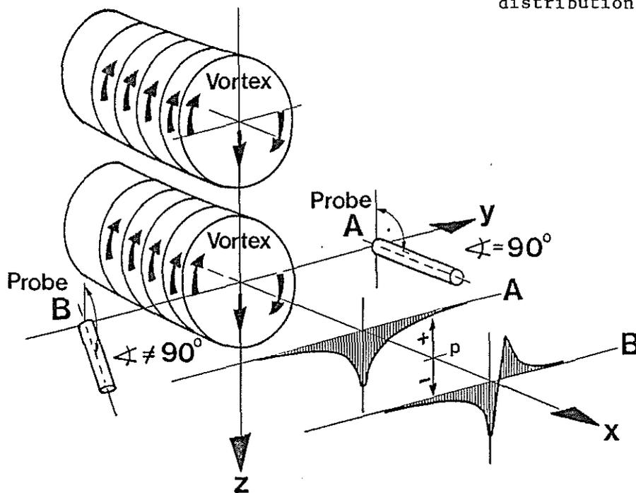
Figure 11. Creation of the two vortex signals
