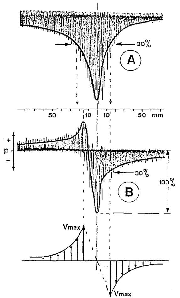
Figure 10. Two different measured pressure signals and a theoretical velocity distribution of a vortex
