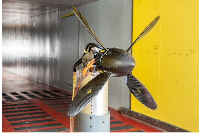
Figure 1. NASA's eVTOL Propeller Icing Test Stand Installed in the Icing Research Tunnel
