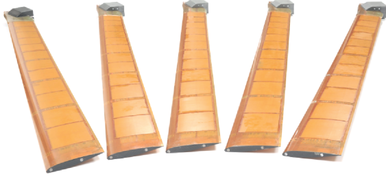
Figure 1: Active twist model rotor blades with MFC actuators
