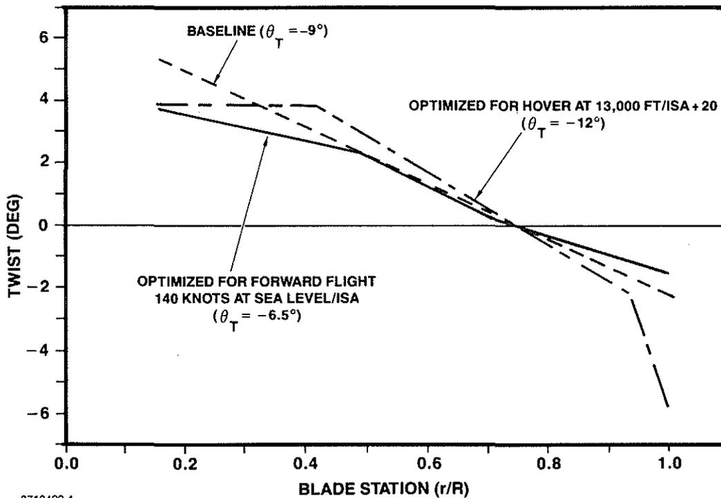
Figure 12. Optimized Main Rotor Blade Twist for a Future Light Helicopter
