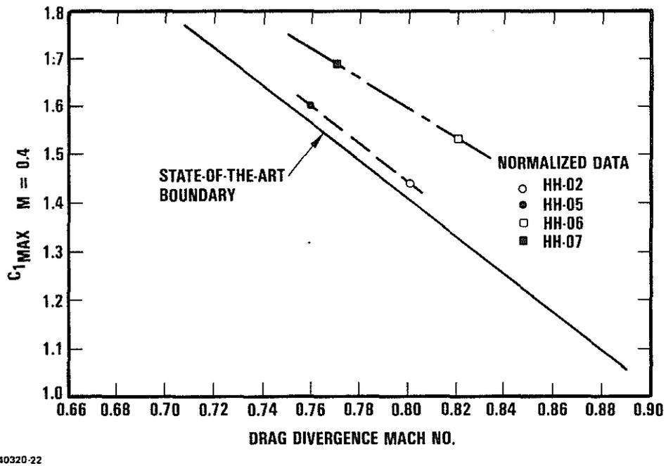
Figure 9. Airfoil  $C_{1MAX}$  Vs Drag Divergence Mach Number
