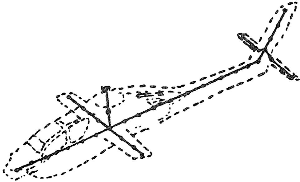
Figure 16. Elastic line Model of AH-64 Fuselage
