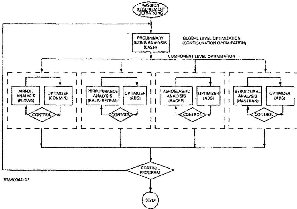
Figure 2. Multilevel Optimization Approach in Helicopter Design
