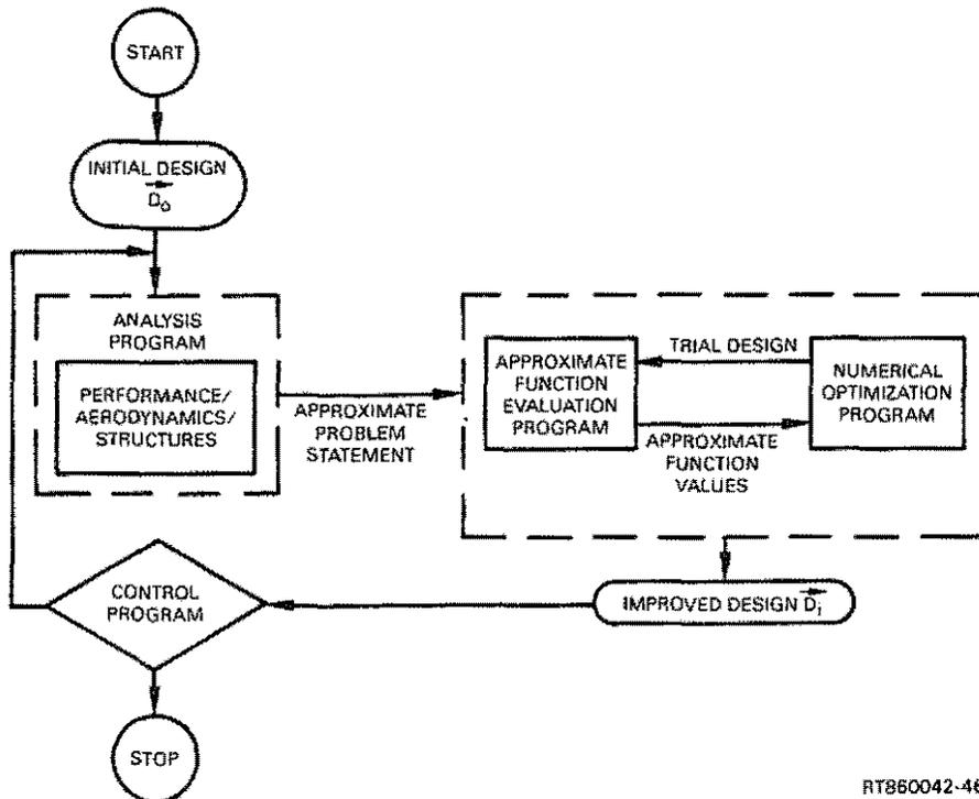
Figure 3. Basic Architecture of the Design Optimization Program
