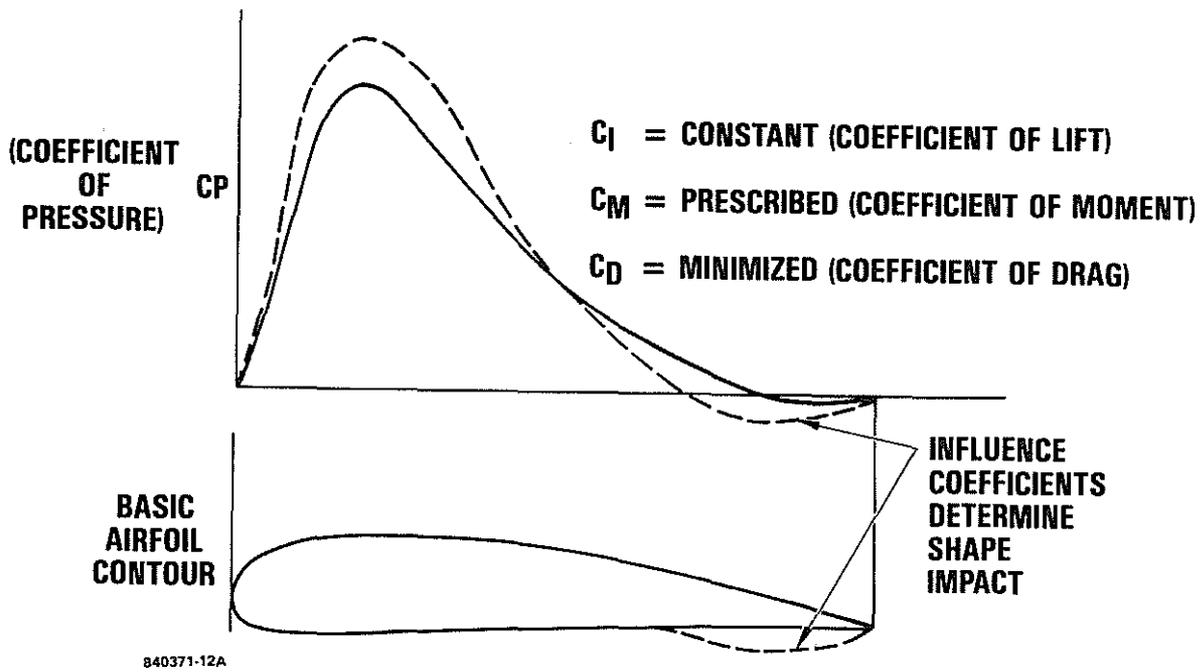
Figure 8. Airfoil Contours and Pressure Distribution
