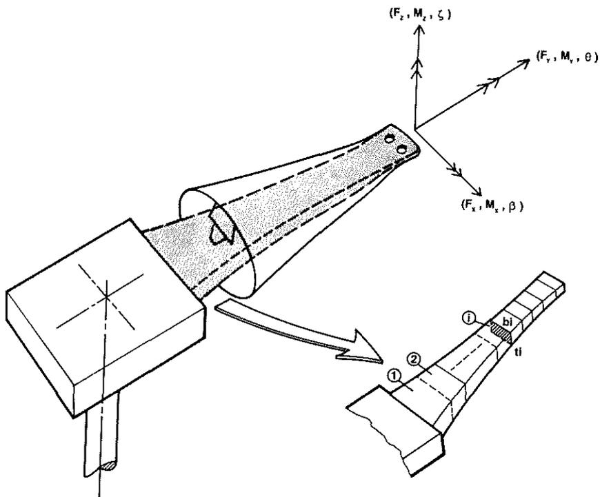
Figure 19. Schematic of Bearingless Main Rotor Hub Model
