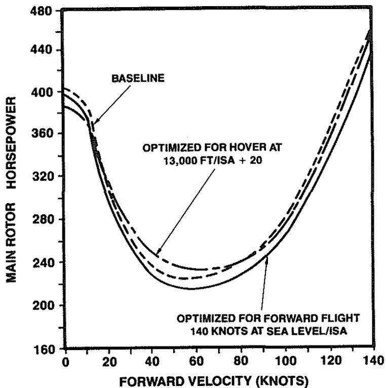
Figure 13. M/R Horsepower Vs Forward Velocity for a Future Light Helicopter
