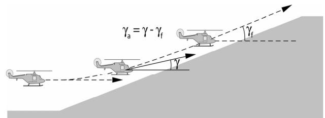
**Fig 10 Flight path angle**
