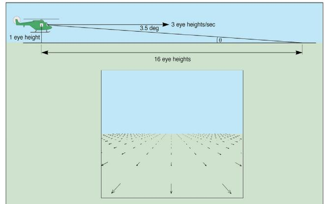
**Fig 1 The optic flow-field and eye-height concept for motion over a flat surface**
