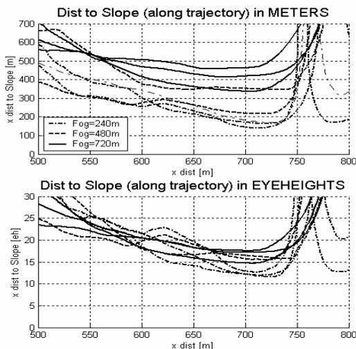
**Fig 8 Distance to the slope surface (in meters and eye-heights)**
