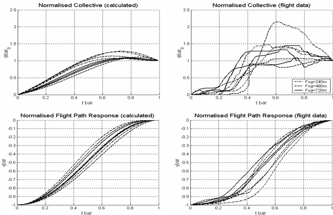
**Fig 16 Comparison of normalised pilot control activity and flight path with  $\tau$ -following strategy**
