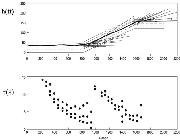
**Fig 4 Variation of height and times to close during terrain hugging manoeuvre**
