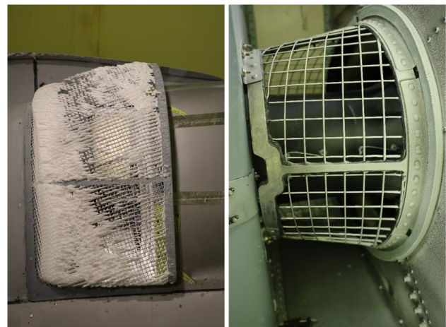
Figure 14: Ice accumulation on grids at -20^{\circ}\text{C}
