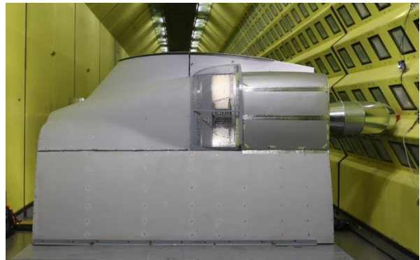
Figure 10: Test model orientation for hover /ground runs
