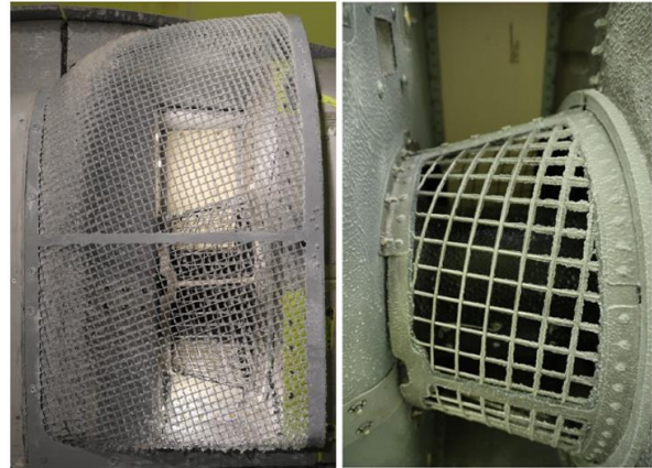
Figure 13: Ice accumulation on grids at -2.5^{\circ}\text{C}
