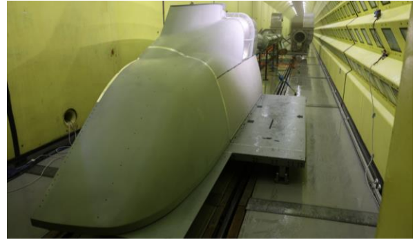
Figure 9: Test model orientation for forward flight
