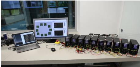
Figure 12: Heater control power supplies and control system setup
