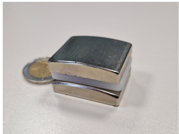
Figure 11: A pair of NdFeB permanent magnets used on the alternator's stator
