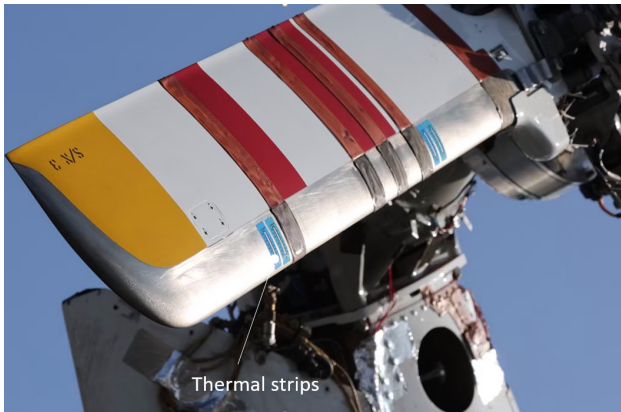
Figure 26: Thermal strips on different blade stations
