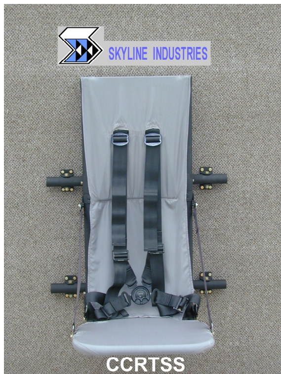
Fig. 13. CCRTSS energy-attenuating troop seat.
