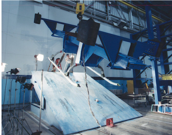
Fig. 19. AH-1Z landing gear drop test.
