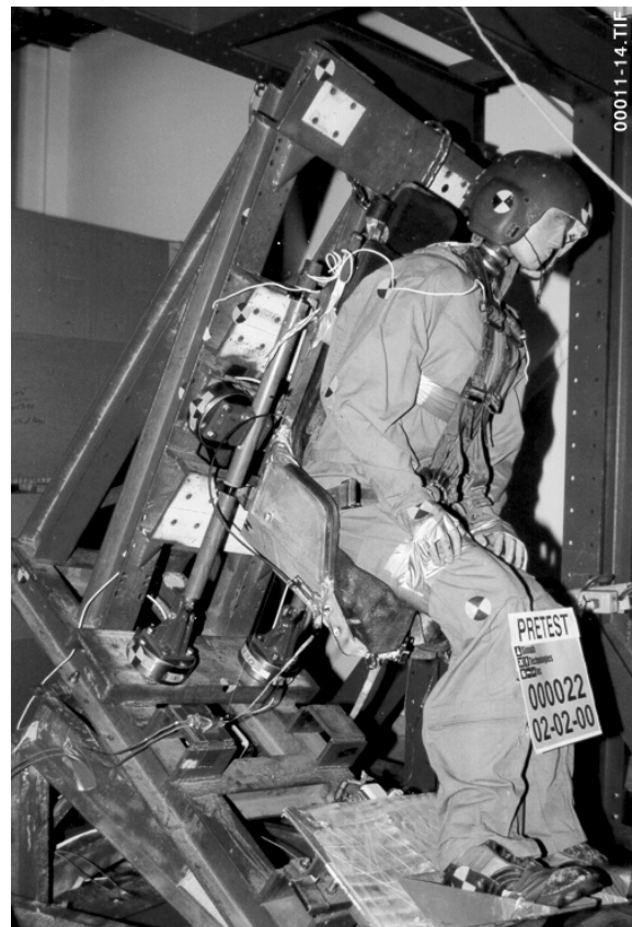
Fig. 18. Crew seat vertical dynamic test.
