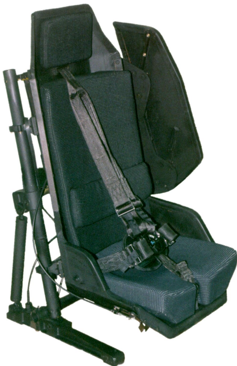
Fig. 17. Common crew energy-attenuating seat.
