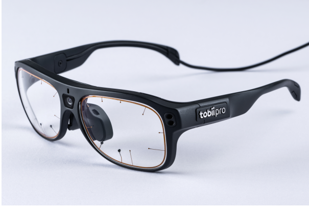
Figure 5. Headworn Eye Tracker Pro Glasses 3 by Tobii
