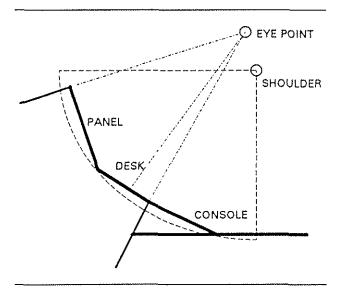
Fig.2 XZ plane cockpit crossection, internal vision and reach layout.
