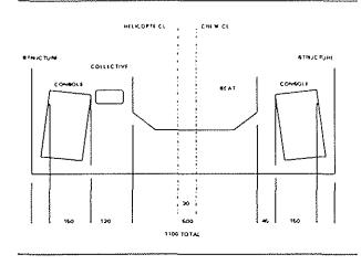
Fig.: 1 YZ plane cockpit cross section, principle
