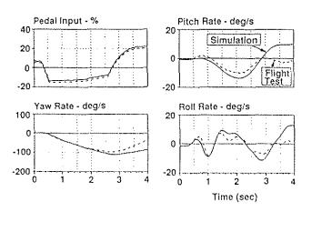
Fig.: 13 Validation of a Hover Turn Manoeuvre
