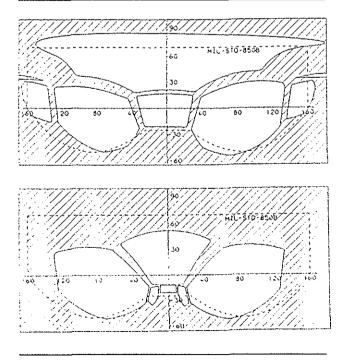
Fig.: 5 Vision Plot forward/rear Cockpit
