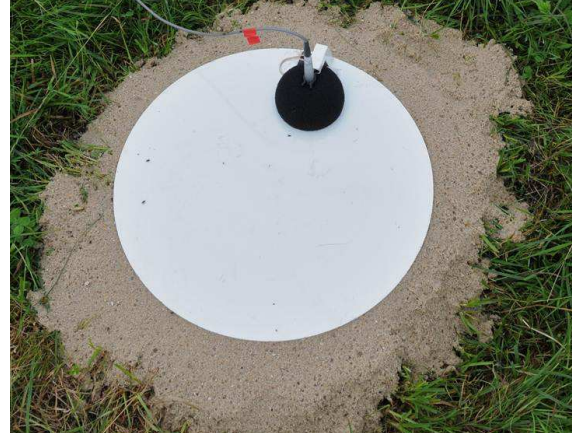
Fig. 2. Installation of considered microphones over a ground plate (GP) for the approach flight.
