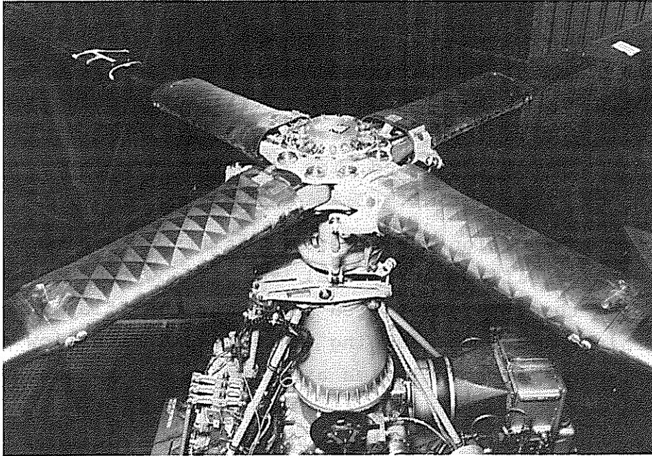
Fig. 7: Bearingless mainrotor for a light helicopter
