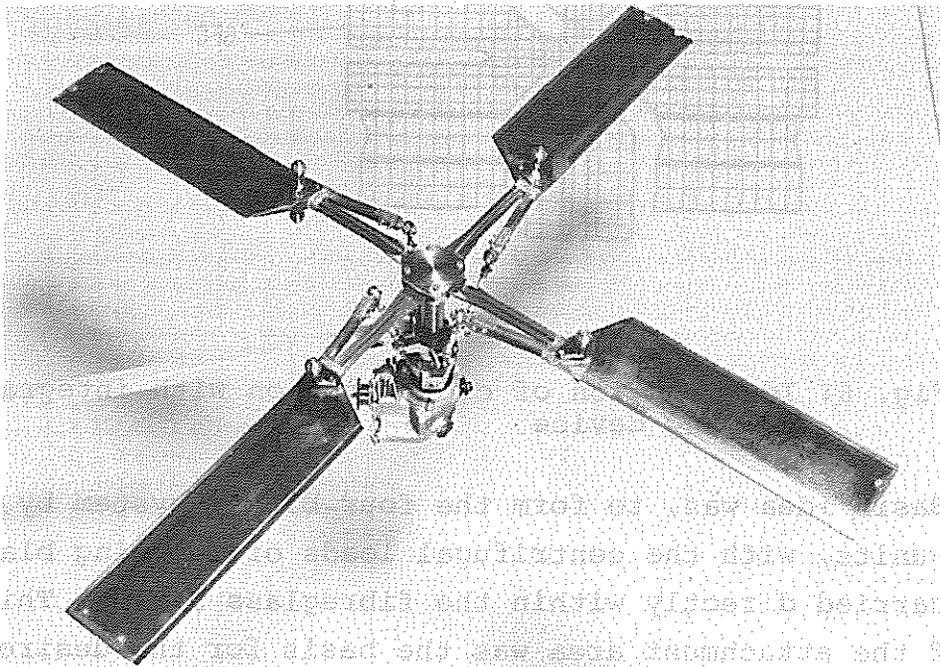
Fig. 5: Bearingless tailrotor
