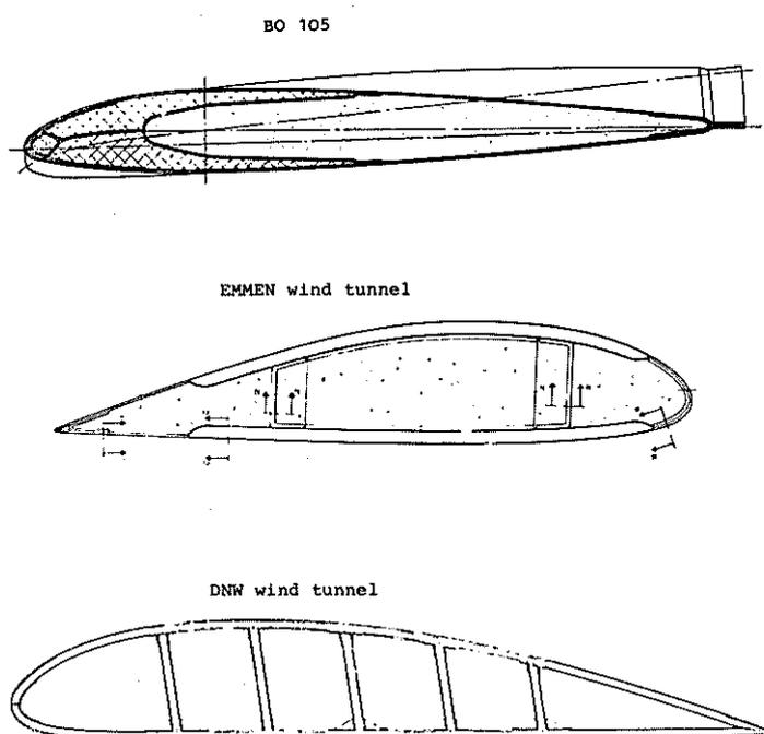
Fig. 11: Cross section of blades
