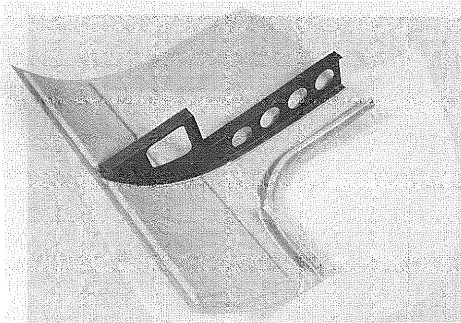
Fig. 27: Side panel with integrated door frame (one shot)
