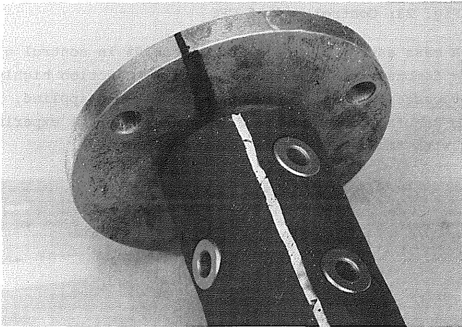
Fig. 22: Load introduction to control tube with collar bushes
