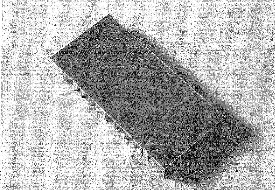
Fig. 3: Wrinkling failure mode of sandwich fibre composite sample due to compression
