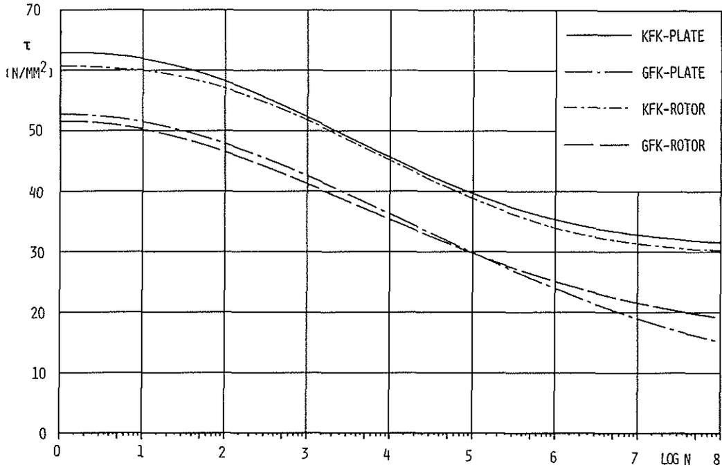
Fig. 2: SN-curves of GFC and CFC samples with the optimized curing and out of rotor hub plates
