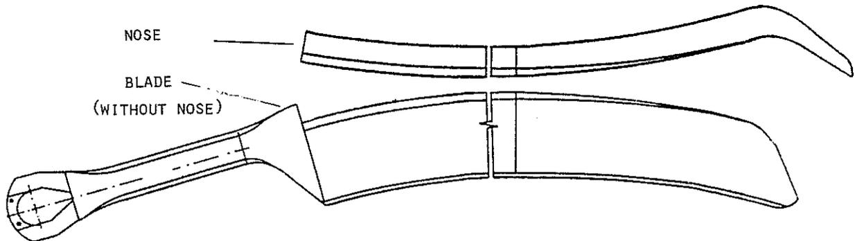
Fig. 12: Leading edge and rest of blade after separate curing cycle before bending together
