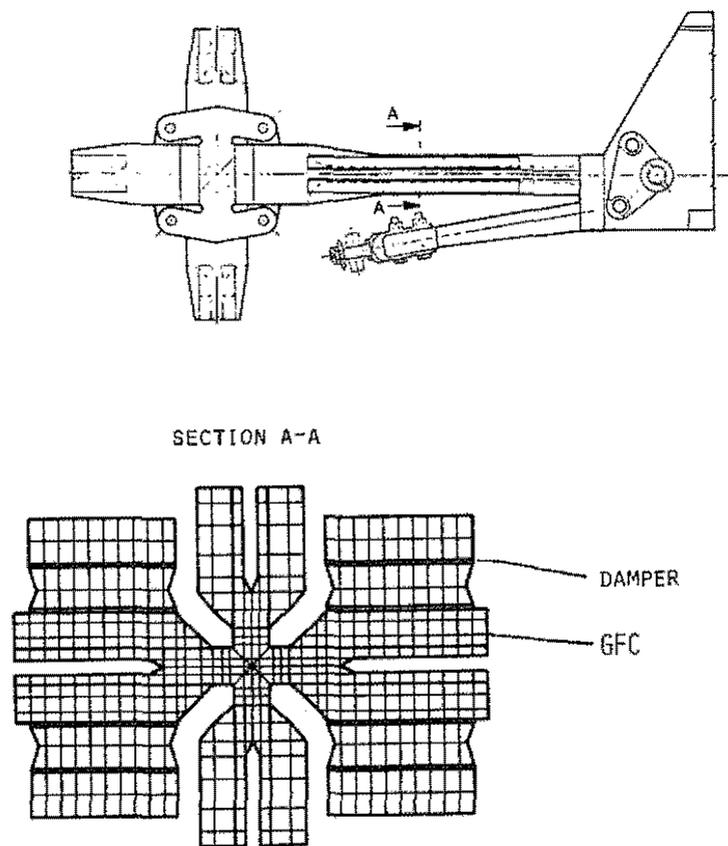
Fig. 6: Idealization of cross section with integrated damping device
