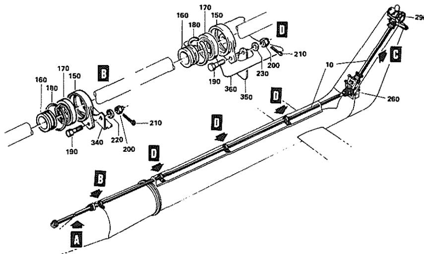
Fig. 17: Drive shaft system of the BO 105
