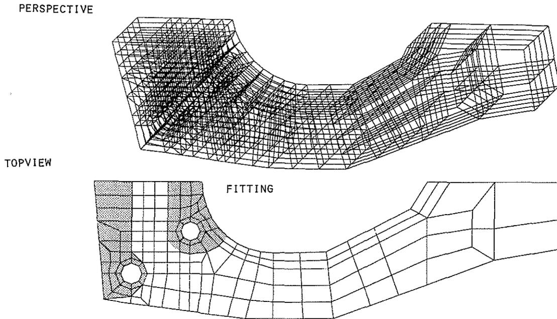
Fig. 13: FEM idealization of root attachment
