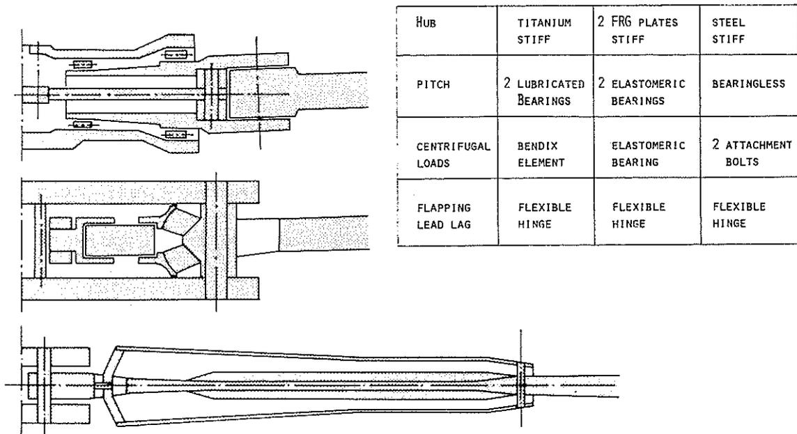
Fig. 10: Comparison of different rotor systems
