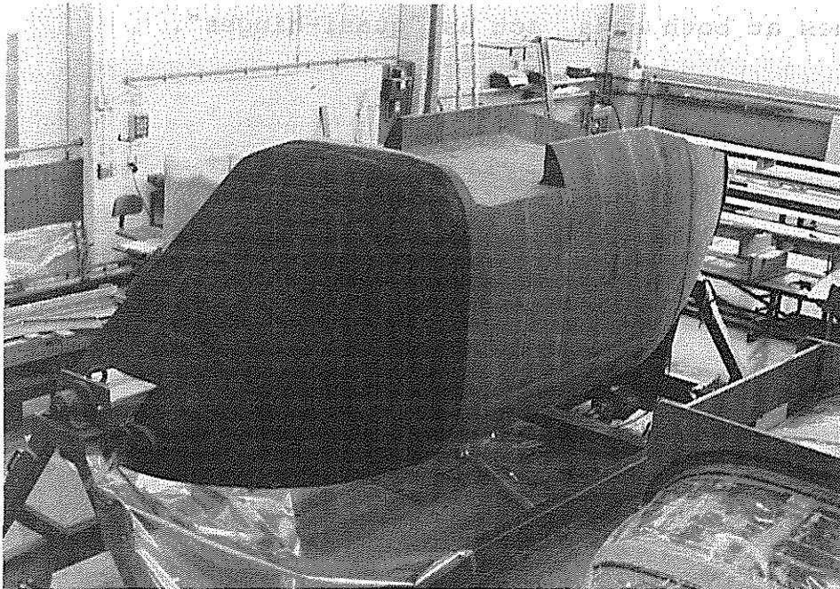
Fig. 26: Master pattern model of all-composite fuselage
