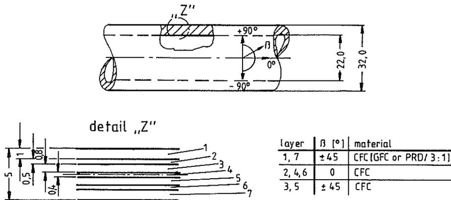
Fig. 18: Typical lay-up for drive shafts
