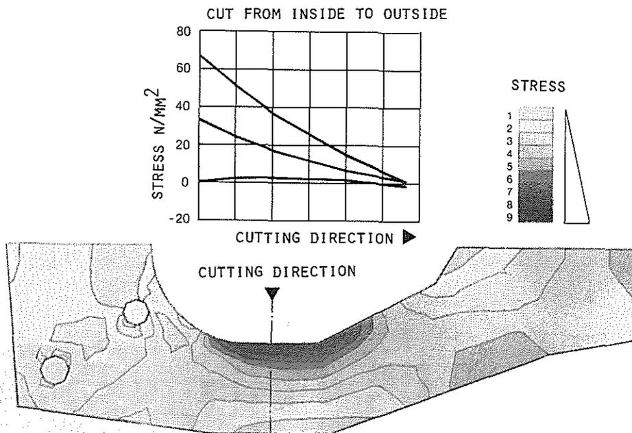
Fig. 14: Stress distribution due to centrifugal load
