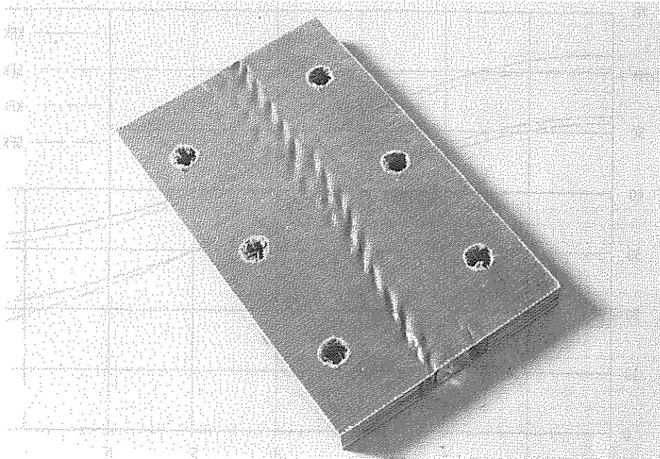
Fig. 4: Wrinkling failure mode of sandwich fibre composite sample to to in-plane shear
