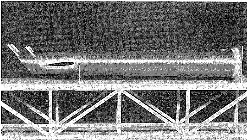
Fig. 28: Filament wound tail boom
