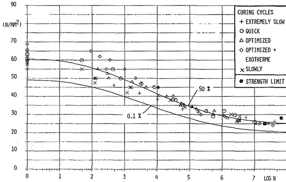
Fig. 1: SN-curve measured with samples with various curing cycles
