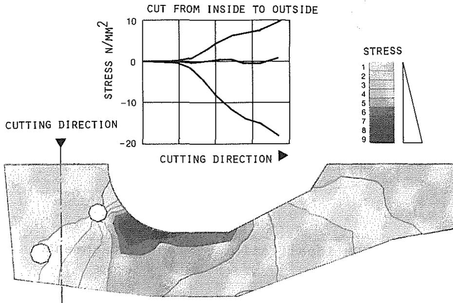
Fig. 15: Stress distribution due to flap bending
