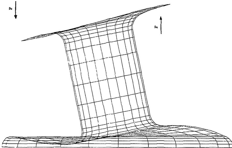
Fig. 19: FEM (half-model) of composite coupling
