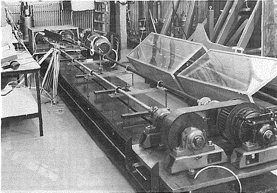
Fig. 20: Long drive shaft on endurance test stand
