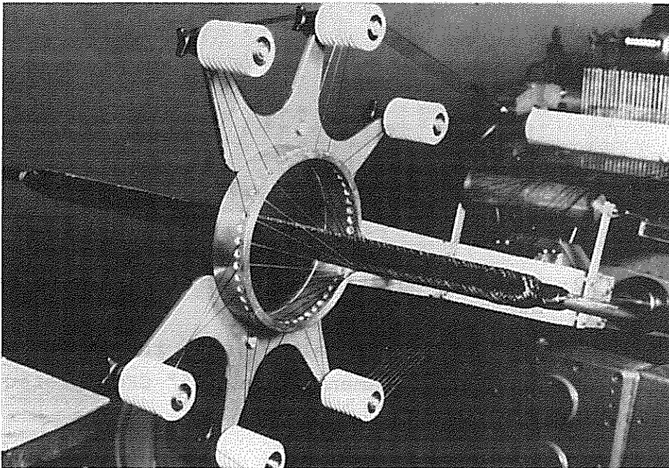
Fig. 24: Filament winding with ring device
