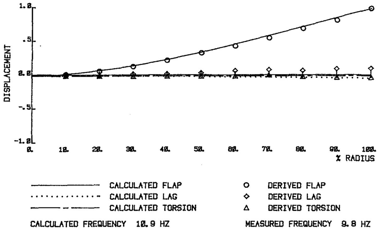
Fig 5 Test Mode 1 Rotor speed 8 rev/s
