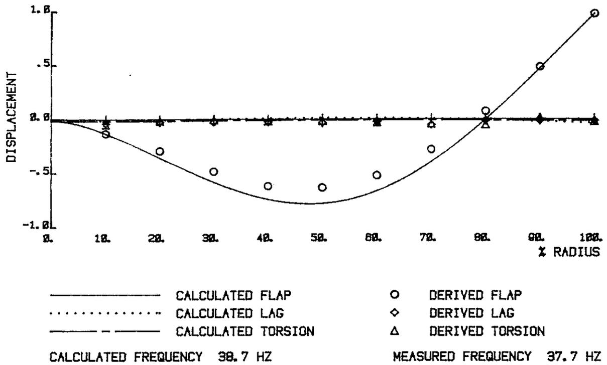
Fig 7 Test Mode 3 Rotor speed 8 rev/s
