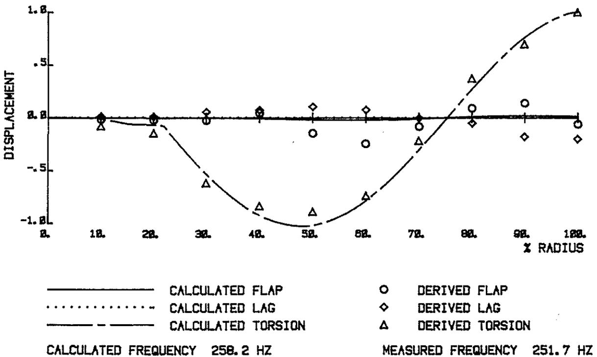
Fig 12 Test Mode 8 Rotor speed 8 rev/s
