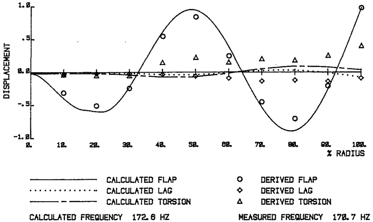
Fig 11 Test Mode 7 Rotor speed 8 rev/s
