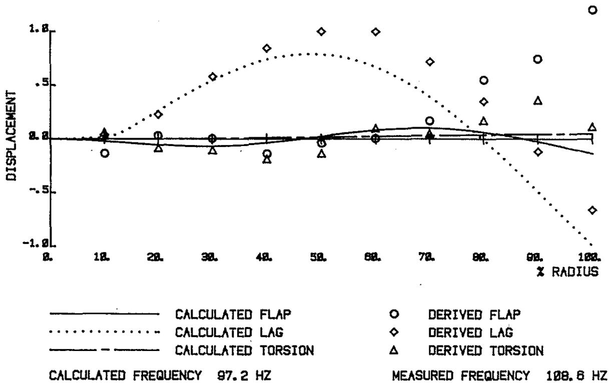
Fig 10 Test Mode 6 Rotor speed 8 rev/s
