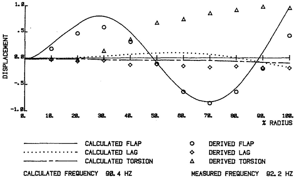
Fig 9 Test Mode 5 Rotor speed 8 rev/s
