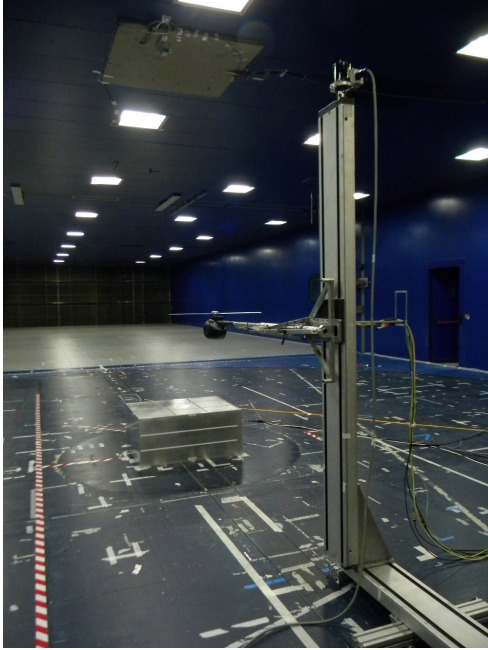
Figure 4: The rotor-obstacle test rig mounted inside the GVPM wind tunnel
