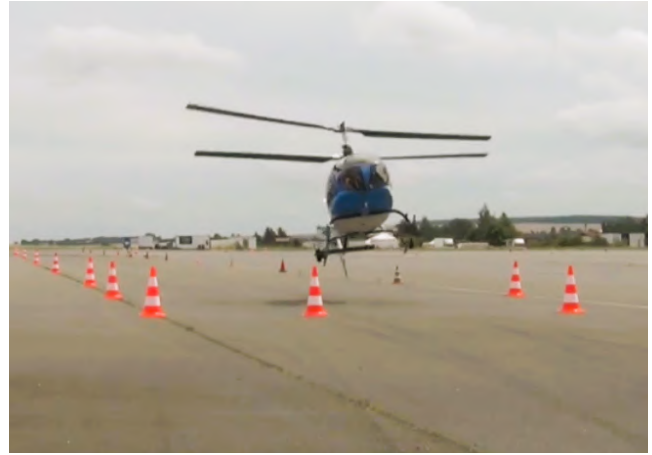
Figure 2: CoAX2D during Acceleration/Deceleration MTE evaluation [2]. Cones and ground markings are used as visual cues.
