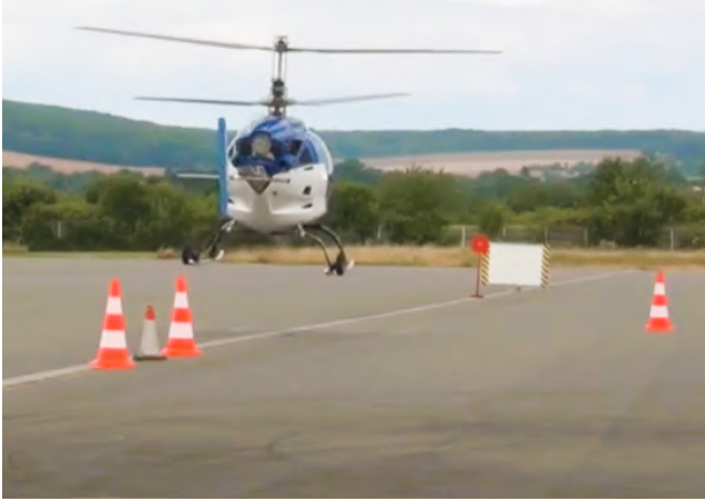
Figure 1: CoAX2D during Hover MTE evaluation [2]. Hoverboards, cones, and ground markings are used as visual cues.
