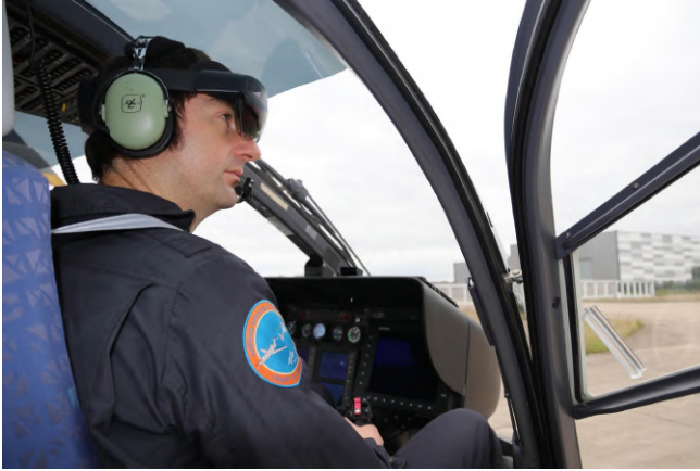
Figure 3: Microsoft HoloLens 2 as HMD in DLRs ACT/FHS cockpit
