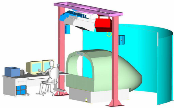
Fig. 2 - FNPT main components – design office drawing
