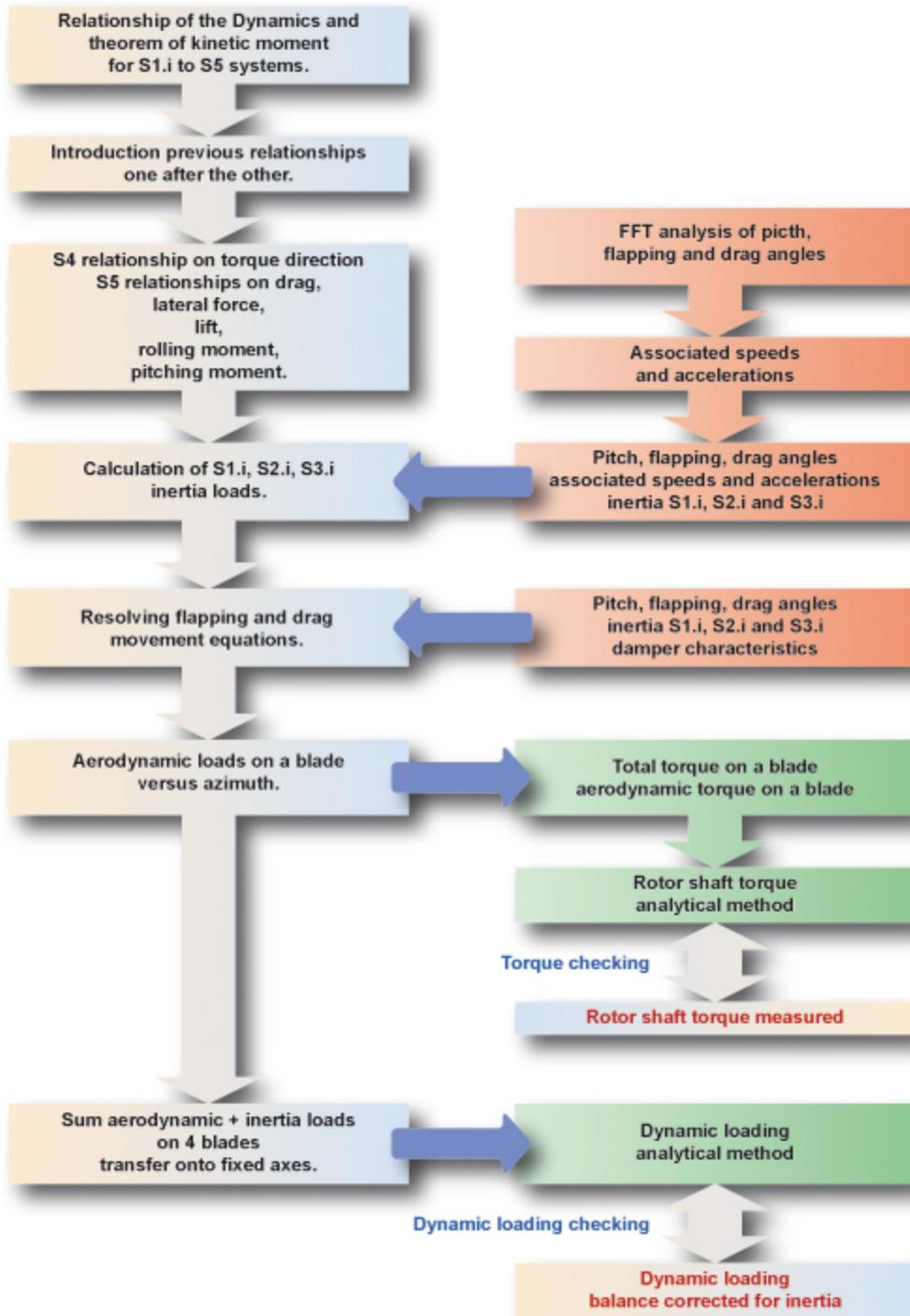
**Fig. 6: Descriptive Flowchart of the Analytical Method**
