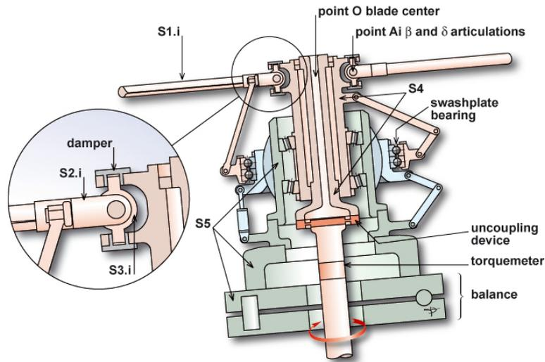
**Fig. 3: Undeformable systems considered by the analytical method**
