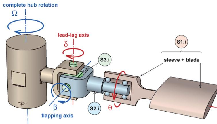
**Fig. 4: Degrees of freedom between systems S1.i, S2.i and S3.i**
