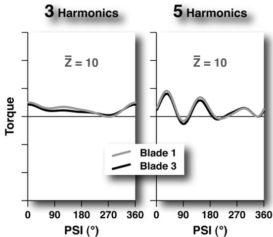
**Fig. 13: Aerodynamic torque on a blade "Modane" control - Calculations up to 3<sup>rd</sup> and 5<sup>th</sup> harmonic**
