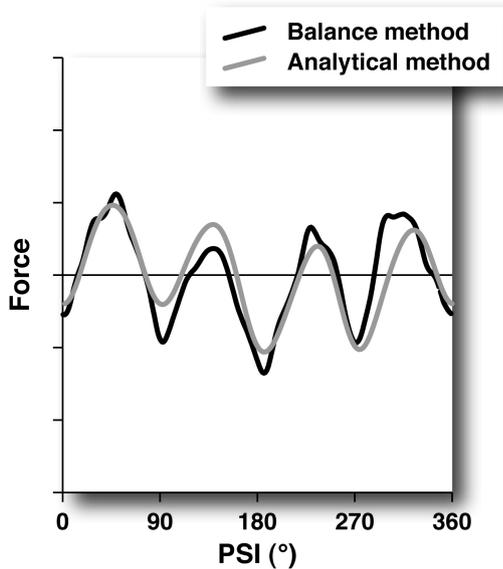
**Fig. 17: Dynamic loading - Lift loads – Analytical method / balance corrected for inertia**
