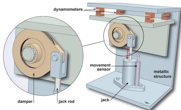
**Fig 9: Diagram of lead-lag damper bench**
