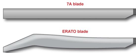
**Fig. 2: Top view of 7A and ERATO blades**
