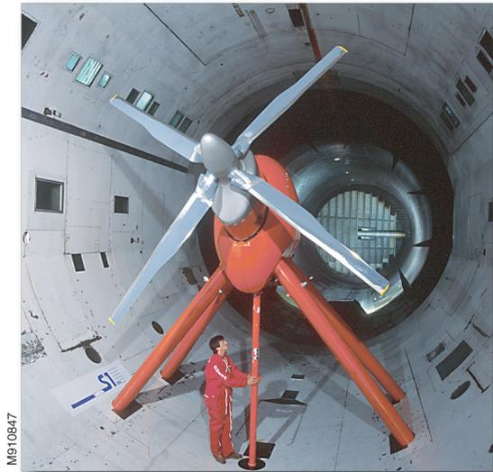
**Fig. 8: ONERA Helicopter Rotor Test Bench in the S1 Modane Windtunnel**
