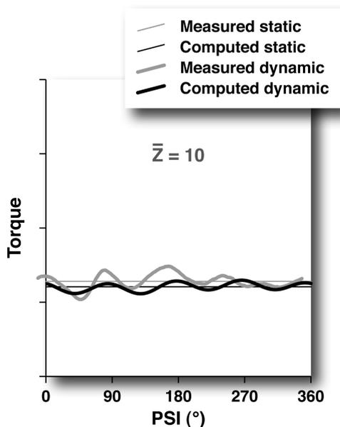
**Fig. 11: Comparison rotor torque calculated / measured**
