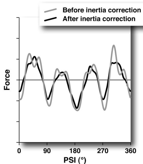
**Fig. 15: Dynamic loading - Rotor lift loads before and after corrections for inertia**
