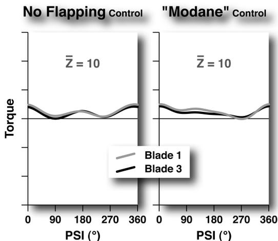
**Fig. 14: Aerodynamic torque on a blade - No flapping / Modane pitch control**
