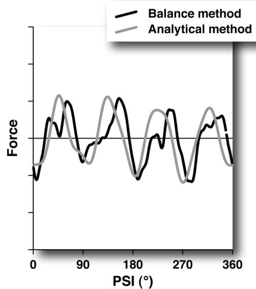
**Fig. 18: Dynamic loading – Rotor drag loads – Analytical method / balance corrected for inertia**
