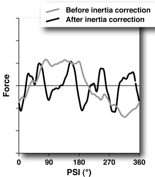
**Fig. 16: Dynamic loading - Rotor drag loads before and after corrections for inertia**
