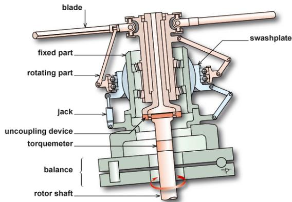
**Fig. 1: Diagram of S1 Modane articulated helicopter rotor**
