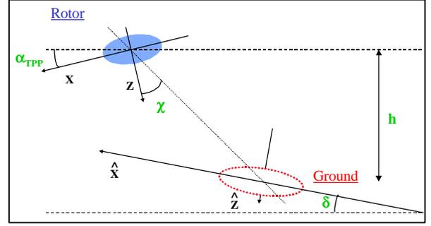
**Figure 11:** helicopter-, wake- and inclined ground frame
