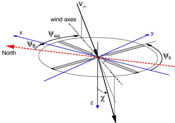
**Figure 4:** reference frame and angle definition
