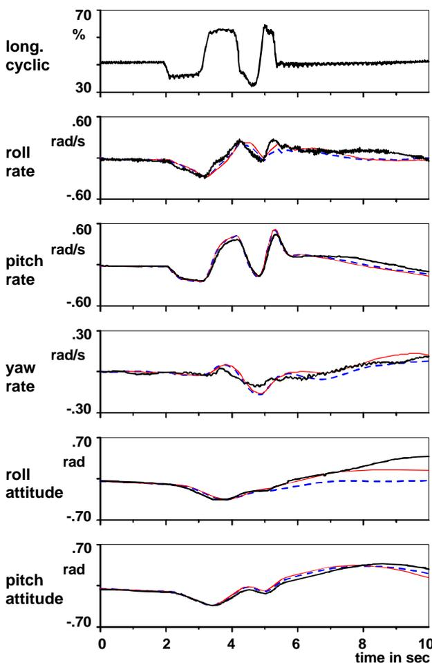
**Figure 6:** longitudinal 3-2-1-1 for BO105 at 100 kts
