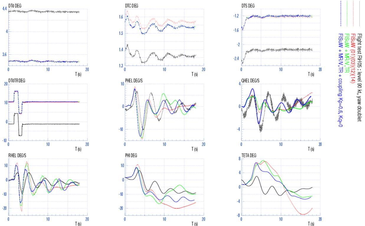
**Figure 9:** Dutch-roll motions after a doublet pedal input for the Dauphin in level flight at 90 kts
