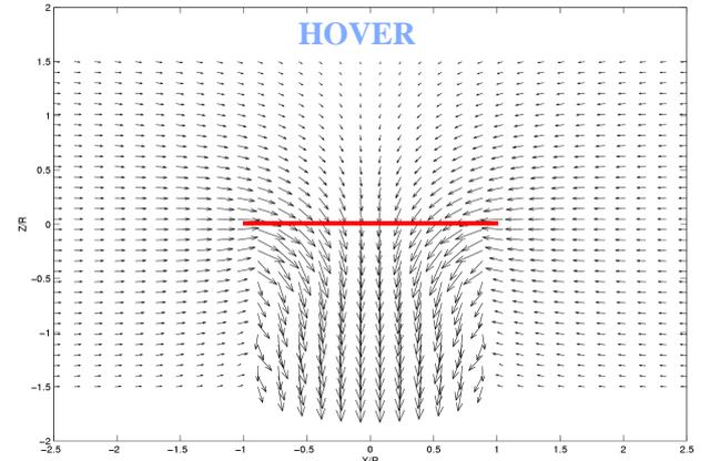
**Figure 7:** induced velocity field of a hovering rotor
