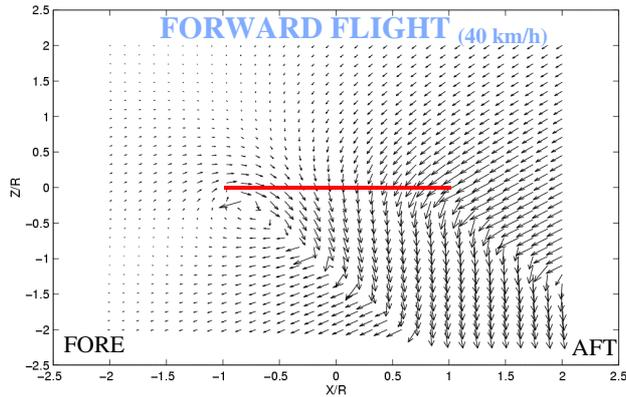
**Figure 8:** induced velocity field in forward flight
