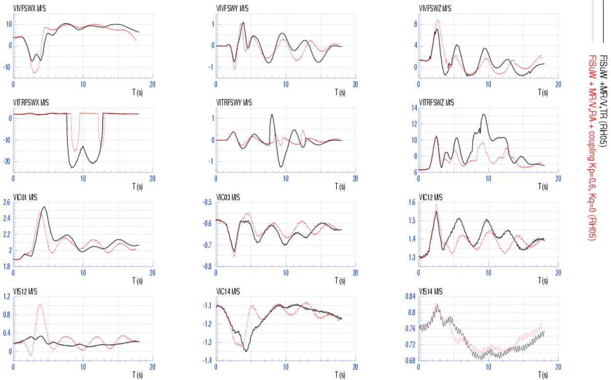
**Figure 10:** induced velocities on fin (ViV\_FSW), tail rotor (ViTR\_FSW) and main rotor, Dauphin at 90 kts
