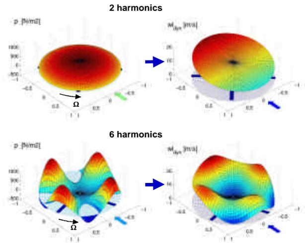
**Figure 1:** pressure and inflow distribution for EC135 at 10 m/s
