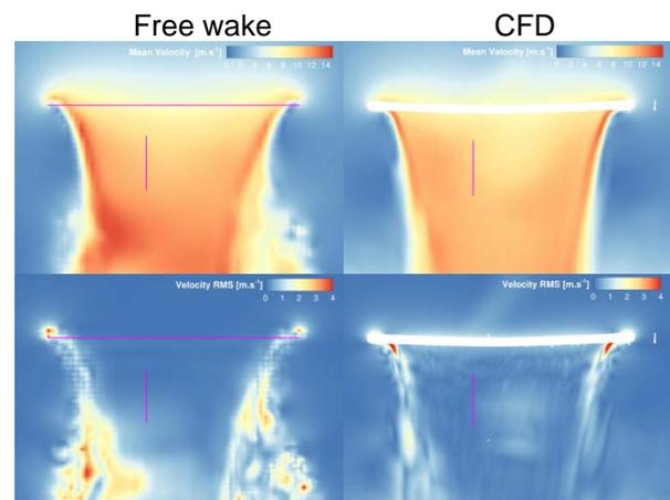
Figure 20: Mean and RMS velocity in a plane passing through the propeller center for isolated rotor in hover
