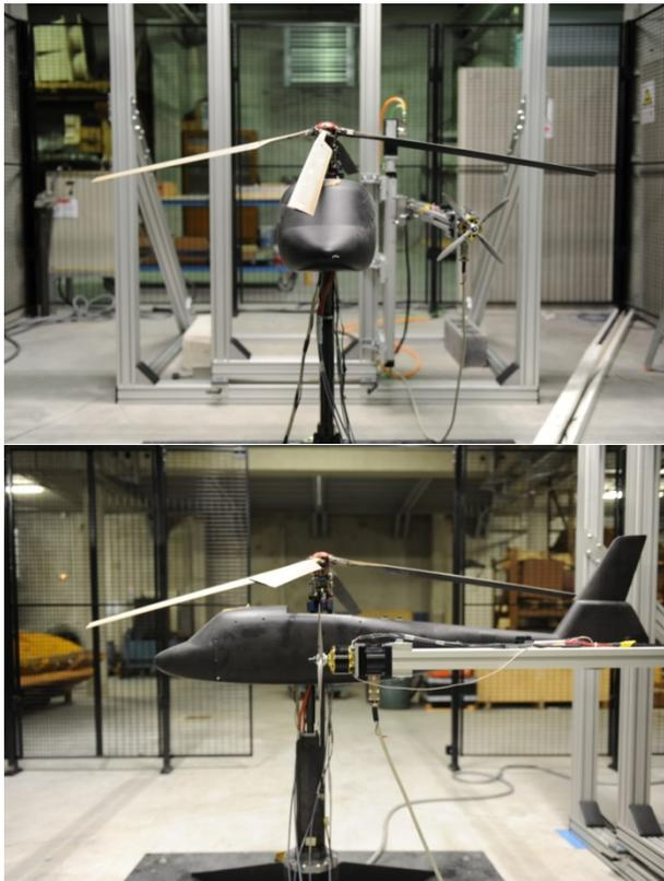
Figure 4: ONERA test rig for Rotor / Propeller wake interaction study
