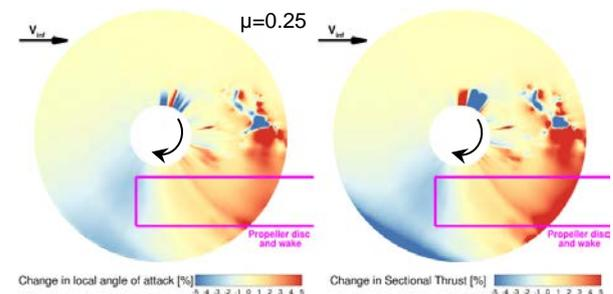
Figure 13: Change in rotor thrust due to the propeller for advance ratio 0.25 using free wake approach.
