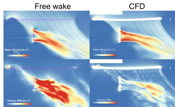
Figure 16: Mean and RMS velocity in a vertical plane passing through the propeller center for installed configurations at advance ratio 0.05
