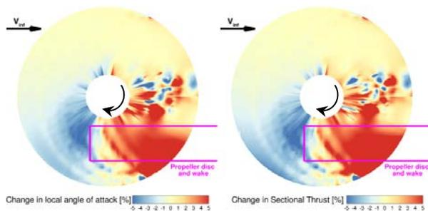
Figure 12: Change in local angle of attack and rotor thrust due the propeller for advance ratio 0.15 using free wake approach.
