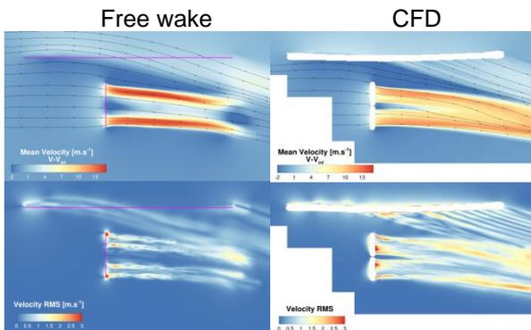
Figure 11: Details of the velocity time average and RMS in rotor and propeller wake at advance ratio 0.15
