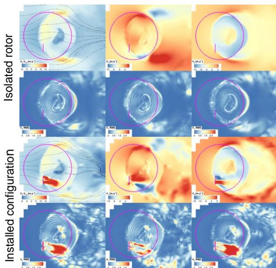
Figure 19: Mean and RMS velocity in an horizontal plane passing through the propeller center at advance ratio 0.05
