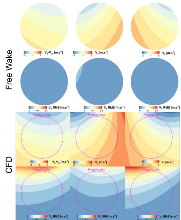
Figure 10: Mean and RMS velocity in the propeller plane for isolated rotor at advance ratio 0.15
