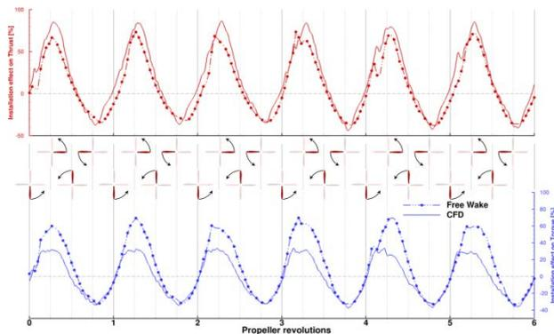
Figure 23: Time history of one propeller blade thrust and power over one rotor revolution (6 propeller revolutions)
