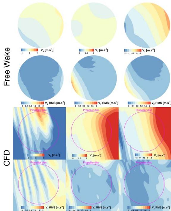
Figure 21: Mean and RMS velocity in the propeller plane for isolated rotor at advance ratio 0.05
