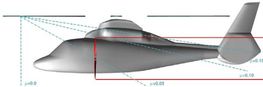
Figure 5: Sketch of isolated propeller and rotor wake path at different advance ratio
