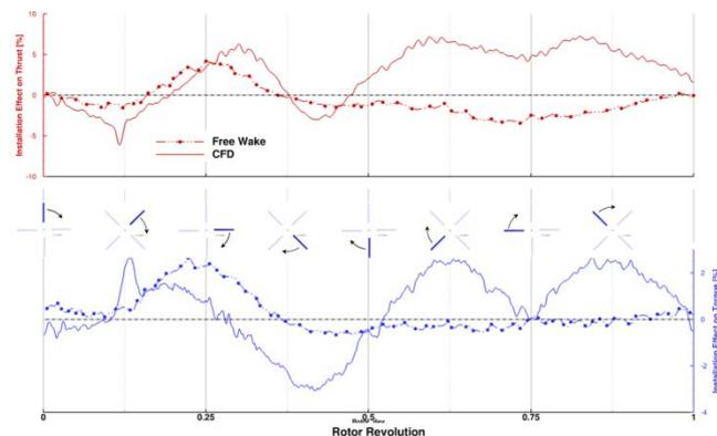
Figure 24: Time history of one rotor blade thrust and power over one rotor revolution
