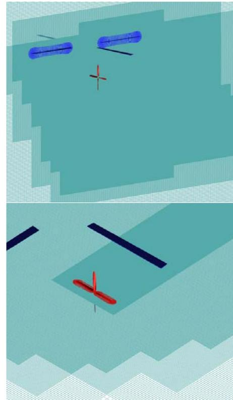
Figure 6: Iso Y (up) and Iso Z (down) view of the CFD mesh for interactional computation at  $\mu=0.05$
