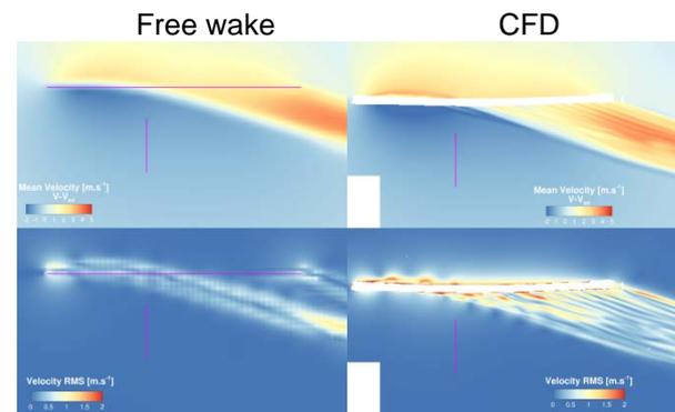
Figure 9: Mean and RMS velocity in a plane passing through the propeller center for isolated rotor at advance ratio 0.15
