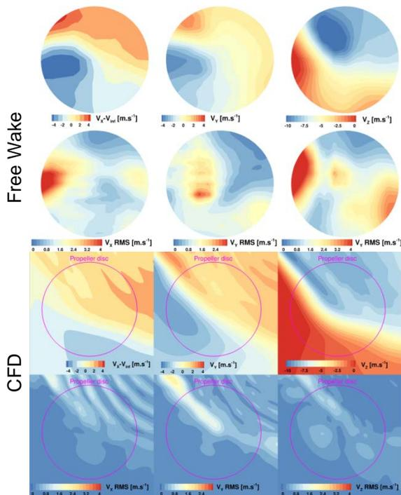
Figure 15: Mean and RMS velocity in the propeller plane for isolated rotor at advance ratio 0.05
