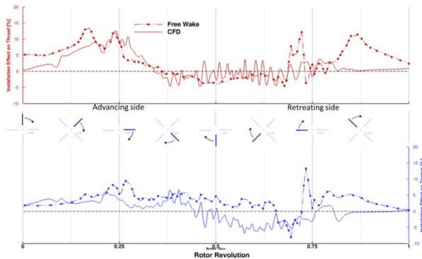
Figure 18: Time history of one rotor blade thrust and power over one rotor revolution
