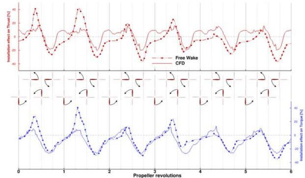
Figure 17: Time history of one propeller blade thrust and power over one rotor revolution (6 propeller revolutions)
