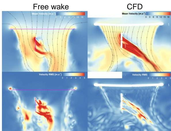
Figure 22: Mean and RMS velocity in a vertical plane passing through the propeller center for installed configuration at advance ratio 0.05
