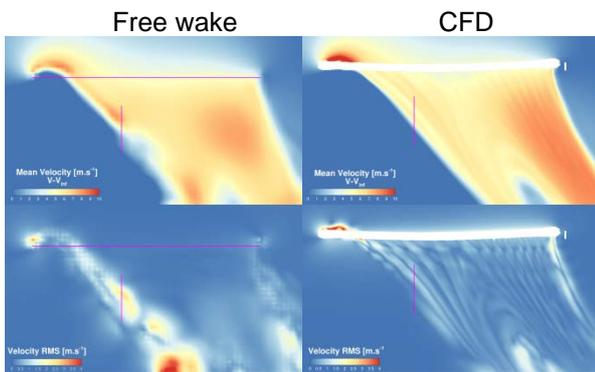
Figure 14: Mean and RMS velocity in a plane passing through the propeller center for isolated rotor at advance ratio 0.05
