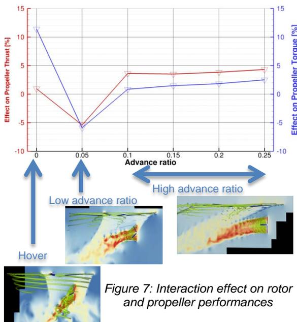
Figure 7: Interaction effect on rotor and propeller performances
