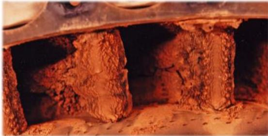
**Figure 2:** HPT NGV damage from molten particulate accumulation<sup>[2]</sup>.
