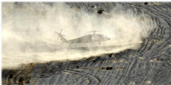
**Figure 1:** Production of a brownout cloud by the UH-60 'Black Hawk' at the Yuma Proving Ground<sup>[1]</sup>.
