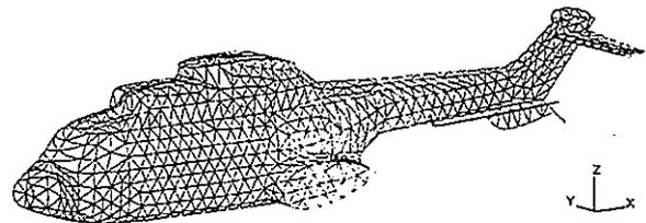
fig. 1 Super Puma mesh for HF application
