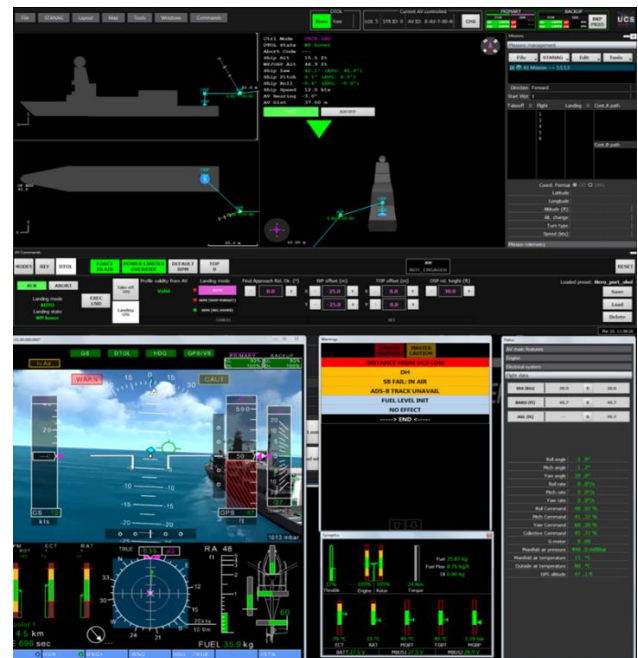
Figure 7: A-UCS displays: AWHERO deck landing simulation (Aircraft at Waiting Point)
