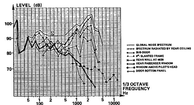
Fig. 15 GLOBAL NOISE SPECTRUM BREAKDOWN FOR REAR PASSENGERS ON BOARD AN SA 365 N FLYING AT 135 kt
