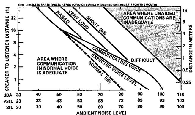
Fig. 2 PERMISSIBLE DISTANCE BETWEEN A SPEAKER AND LISTENERS FOR SPECIFIED VOICE LEVELS AND AMBIENT NOISE LEVELS
