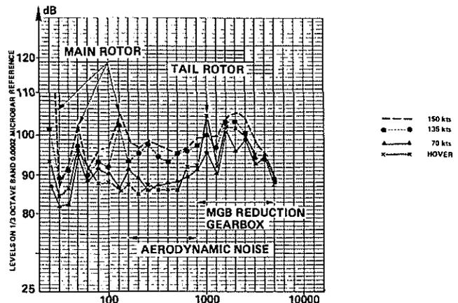
Fig. 7 VARIATIONS OF NOISE SPECTRA IN SA 365 N CABIN VERSUS FLIGHT SPEED AIRCRAFT WITHOUT SOUND-PROOFING - FRONT - PASSENGER
