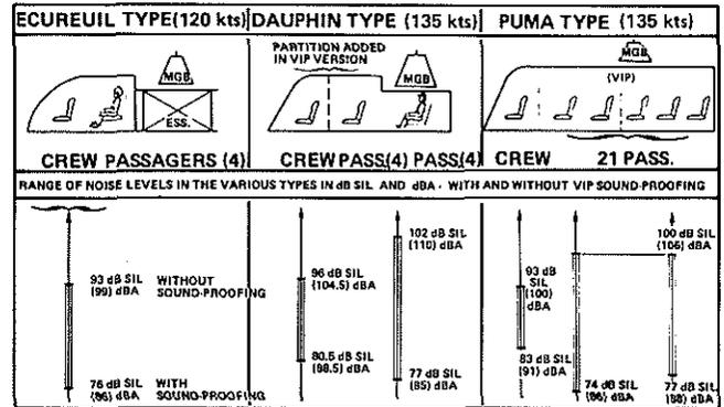
Fig. 1 COMPARING THE VARIOUS TYPES OF HELICOPTERS
