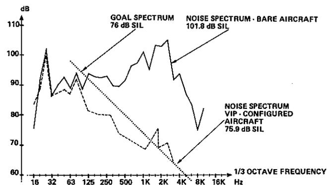
Fig. 31 SA 365 N PASSENGER SEATING IN THE MIDDLE OF REAR CABIN (FLYING AT 135 kt )
