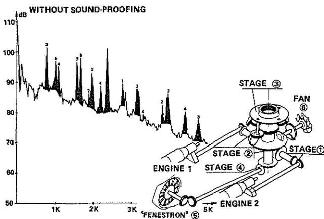
Fig. 4 SA 365 N- INTERNAL NOISE SPECTRUM (PASSENGER SEAT UNDER MGB)
