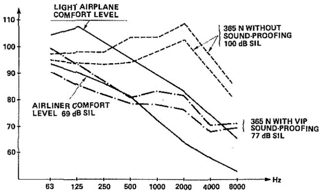
Fig. 3 NOISE SPECTRA AND LEVELS AS MEASURED ON BOARD AN SA 365 N WITHOUT AND WITH VIP SOUND-PROOFING CRUISE FLIGHT: 135 kt
