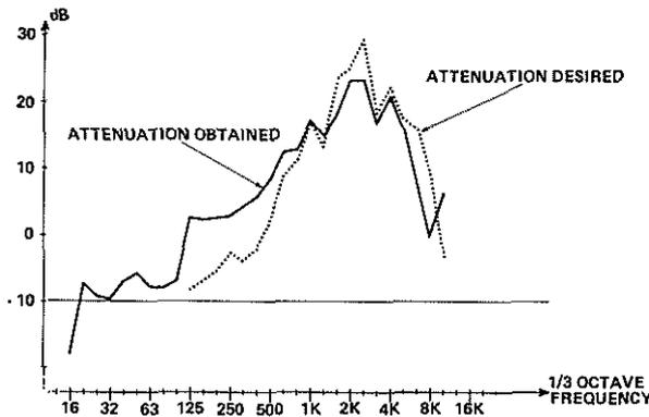
Fig. 33 SA 365 N- PASSENGER SEATING IN THE MIDDLE OF REAR CABIN FLYING AT 135 kt
