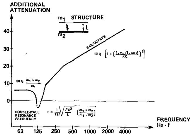
Fig. 32 ATTENUATION FOR AN ADDITIONAL SEPARATE WALL
