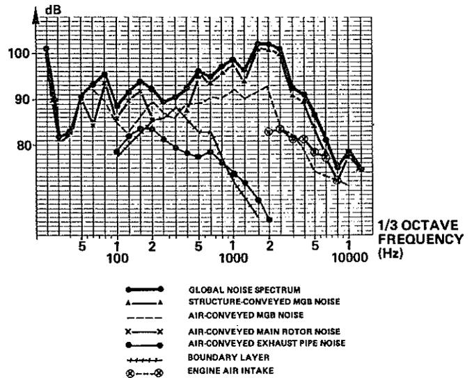
Fig. 14 NOISE SPECTRUM AT REAR OF CABIN SA 365 N 135 kt CRUISE FLIGHT
