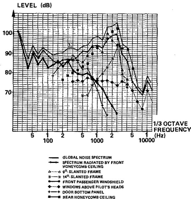
Fig. 16 GLOBAL NOISE SPECTRUM BREAKDOWN FOR FRONT PASSENGERS ON BOARD AN SA 365 N FLYING AT 135 kt
