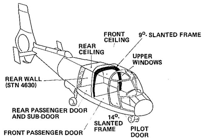
Fig. 5 SA 365 N STRUCTURE COMPONENTS
