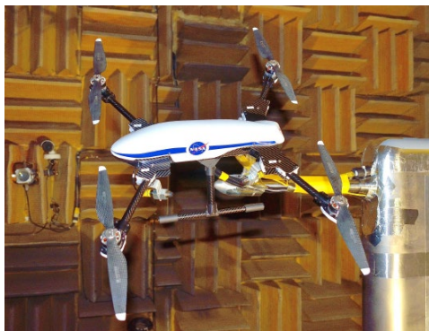
Figure 1. SUI Endurance vehicle installed on Model Test Stand (MTS) in LSAWT (the images taken from Ref. 3).
