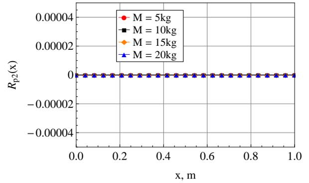
Figure 10: Plot of the residues,  $R_{p1}$  &  $R_{p2}$ , after putting the derived expressions of mass density, shear modulus and elastic modulus, given by Figs. 7, 8 & 9, respectively, of a rotating pinned-free Timoshenko beam into the governing differential equations
