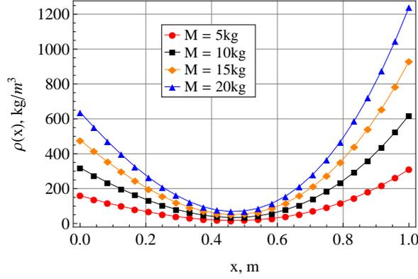
Figure 7: Density variations for a rotating pinned-free Timoshenko beam, for different values of the total mass, whose first mode shape is given by Fig. 6
