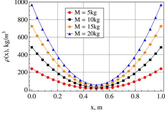
Figure 2: Density variations for a rotating cantilever Timoshenko beam, for different values of the total mass, whose second mode shape is given by Fig. 1
