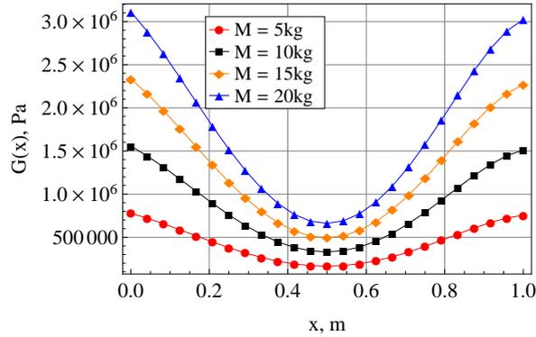
Figure 8: Shear modulus variations for a rotating pinned-free Timoshenko beam, for different values of the total mass, whose first mode shape is given by Fig. 6
