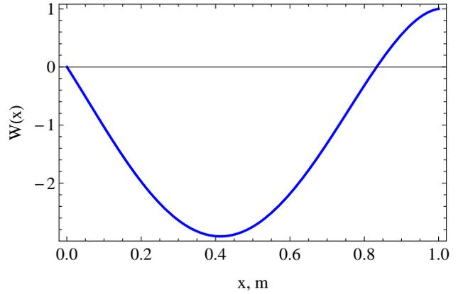
Figure 1: **The assumed mode shape  $W(x)$ , for a rotating cantilever Timoshenko beam second mode**
