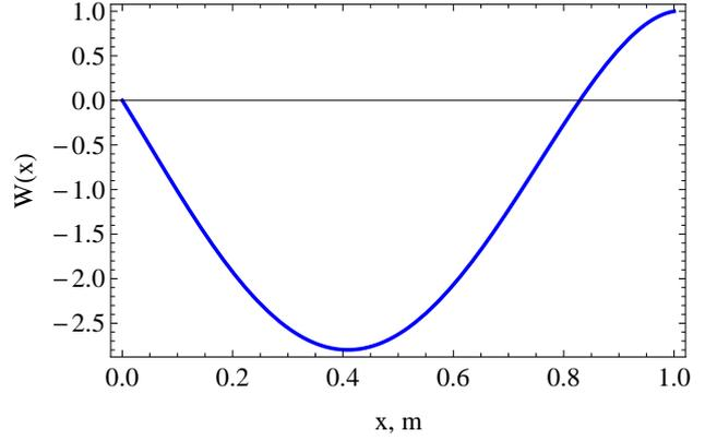
Figure 6: **The assumed mode shape  $W(x)$ , for a rotating pinned-free Timoshenko beam first mode**
