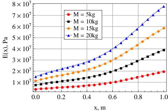
Figure 4: Elastic modulus variations for a rotating cantilever Timoshenko beam, for different values of the total mass, whose second mode shape is given by Fig. 1
