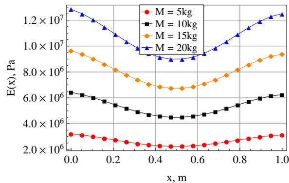
Figure 9: Elastic modulus variations for a rotating pinned-free Timoshenko beam, for different values of the total mass, whose first mode shape is given by Fig. 6
