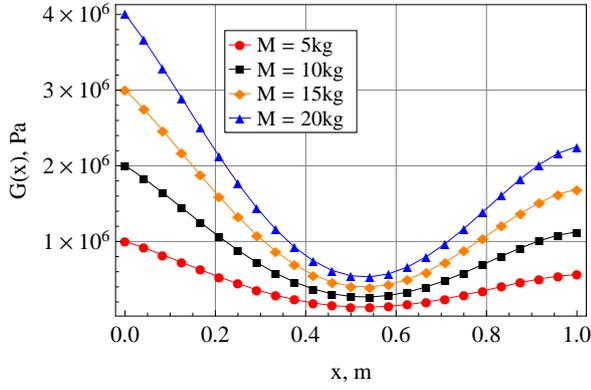
Figure 3: Shear modulus variations for a rotating cantilever Timoshenko beam, for different values of the total mass, whose second mode shape is given by Fig. 1
