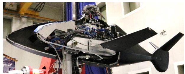
Figure 2: Wind tunnel model inner structure.
