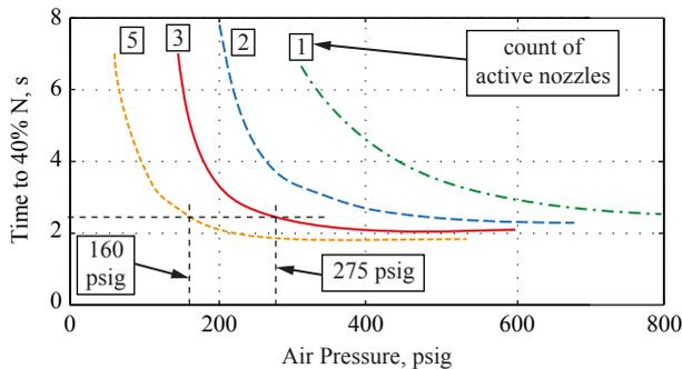
**Figure 3: Start-up time to 40% gas generator speed depending on nozzle count and nozzle pressure [9]**
