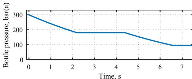
**Figure 7: Bottle pressure of the airworthy QSS preliminary design for two consecutive operations**
