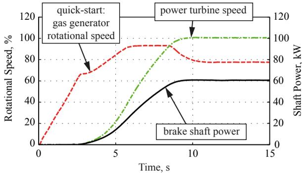
**Figure 2: Quick-start rotational speed of gas generator and power turbine as well as delivered shaft power.**
