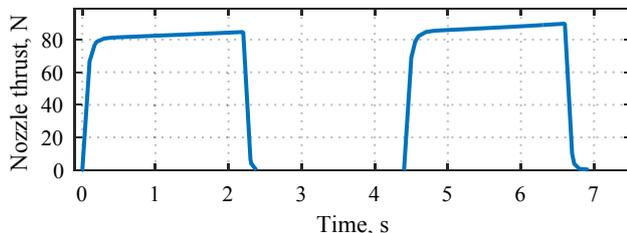
**Figure 6: Thrust of one nozzle of the airworthy QSS preliminary design for two consecutive operations**
