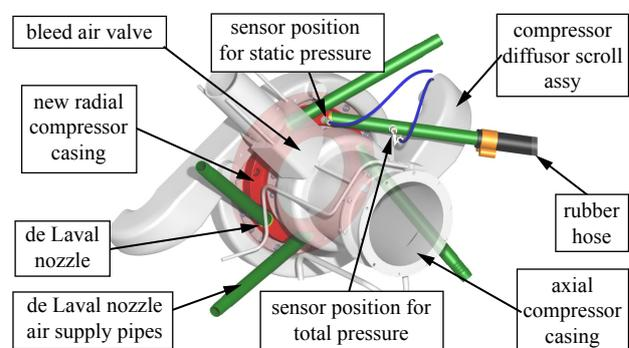
**Figure 1: Integration and positioning of the de Laval nozzles.**
