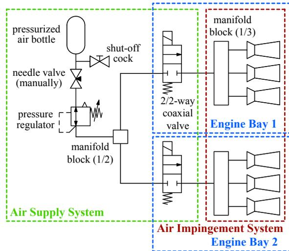
**Figure 4: Scheme of the airworthy quick-start system**
