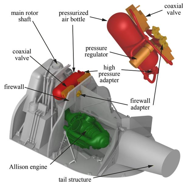
**Figure 8: CAD model of a possible QSS arrangement within the BO 105 fuselage**
