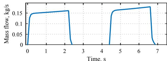
**Figure 5: Mass flow of one nozzle of the airwor. QSS preliminary design for two consecutive operations**
