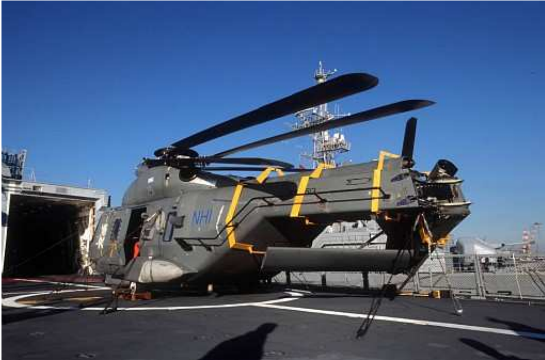
Figure 2 : NFH version – Standard cabin – Folding phase
