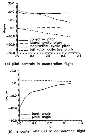
Fig. 4The Pilot Controls and Attitudes of helicopter DOLPHIN from hover to maximum speed
