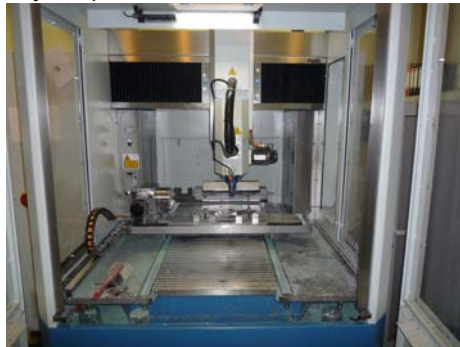
ProfiSpeed 600 Numerical Control milling machine
