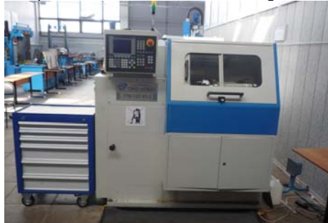
TPK-125A1-1 Numerical Control lathe machine
