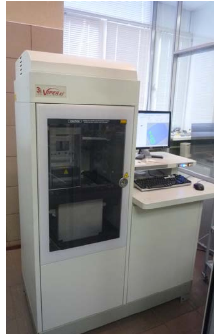
Viper si2TM laser stereo lithography processing machine
