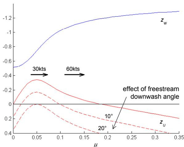
Figure 2. Effect of advance ratio on longitudinal rotor thrust derivatives [10]
