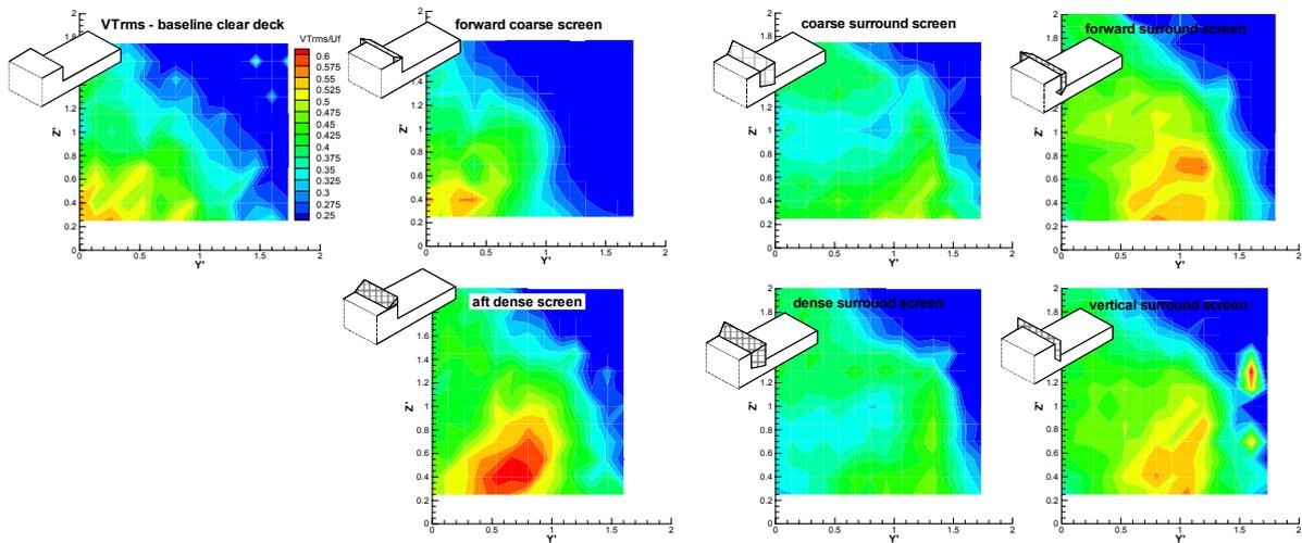
Figure 10. Addition of hangar door side screens to improve lateral turbulence distribution ( $x/L = 1$ )
