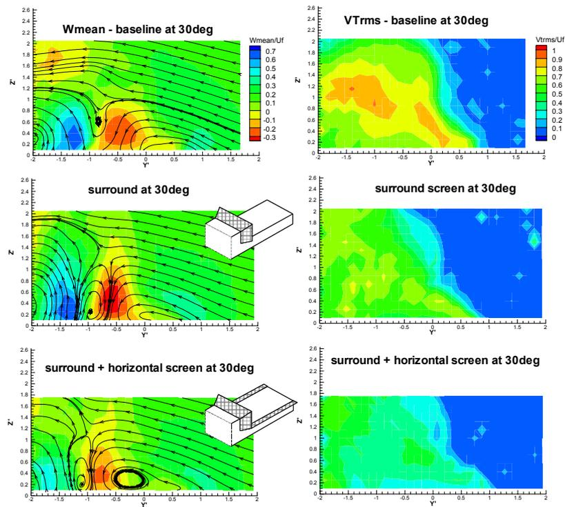
Figure 13. Effect of flight deck edge screens on lateral downwash and turbulence intensity distributions ( $x/L = 1$ )
