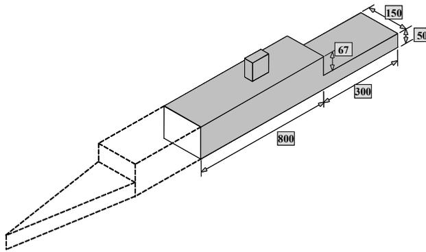
Figure 5. TTCP 'Simplified Frigate Shape'
