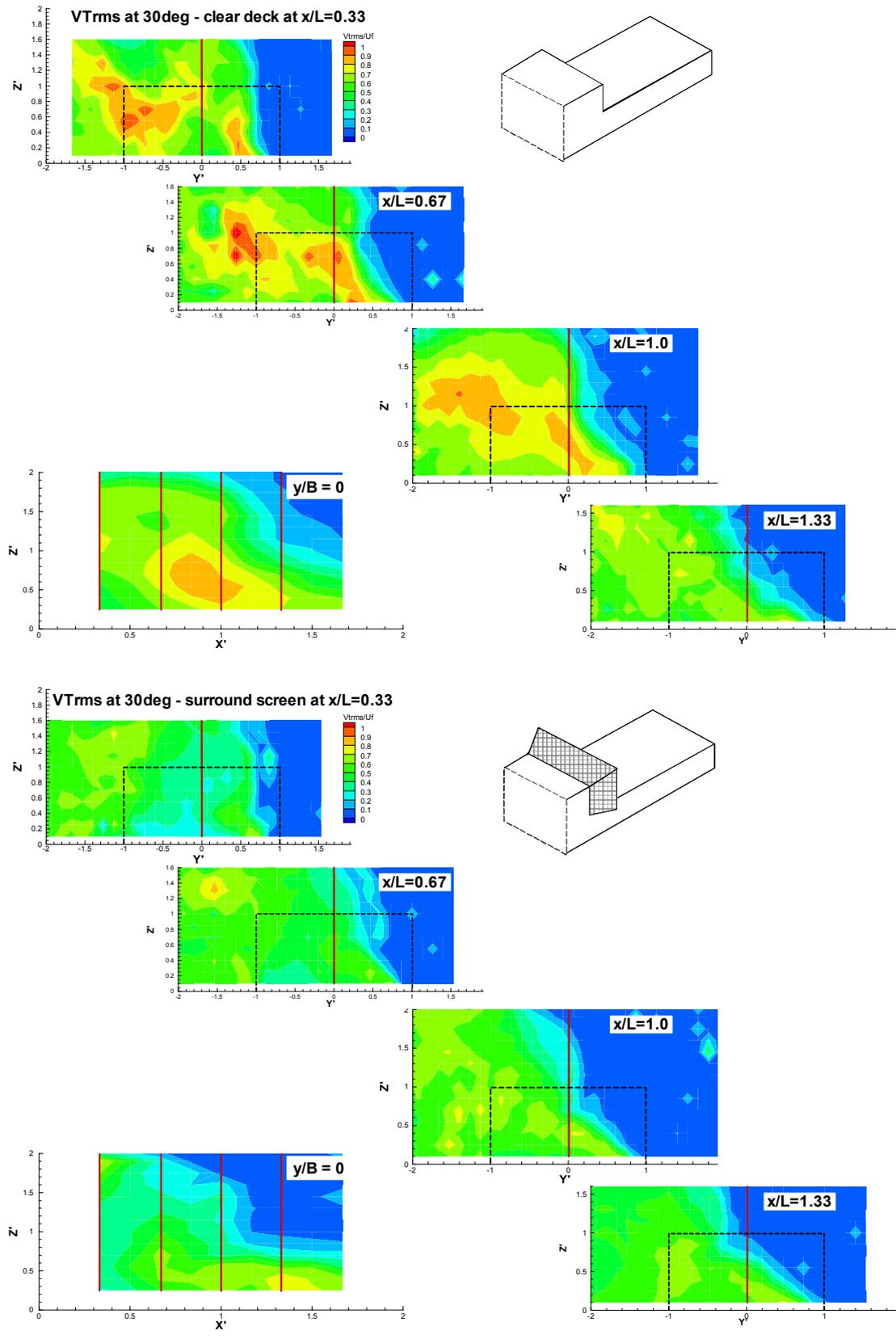
Figure 12. Effect of flow control on turbulence distribution with 30° crosswind
