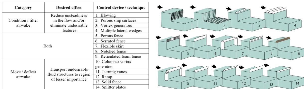
Figure 3. AVT-102 Ship air wake flow control classification [11]
