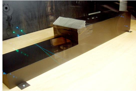
Figure 6. Frigate model with forward-facing 'coarse' hangar roof screen
