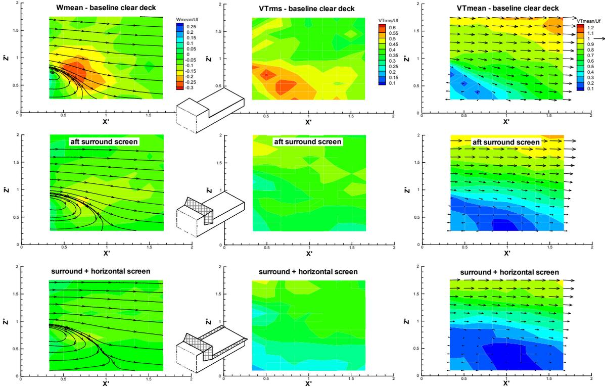
Figure 9. Effect of hangar and flight deck edge screens on longitudinal downwash, turbulence intensity and velocity deficit distributions ( $y/B = 0$ )
