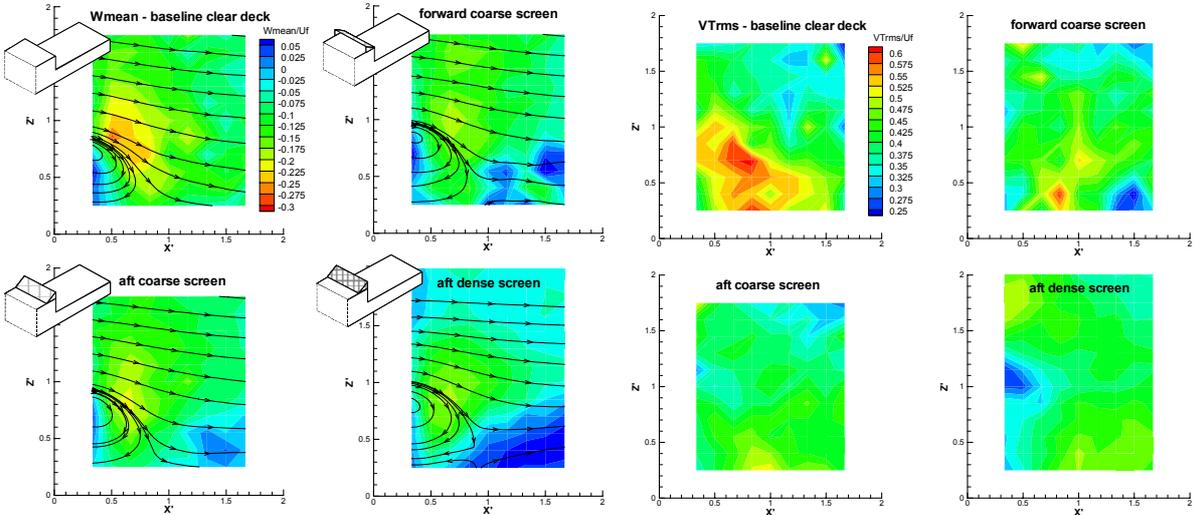
Figure 8. Effect of hangar roof screens on longitudinal distribution of downwash and turbulence intensity ( $y/B = 0$ )
