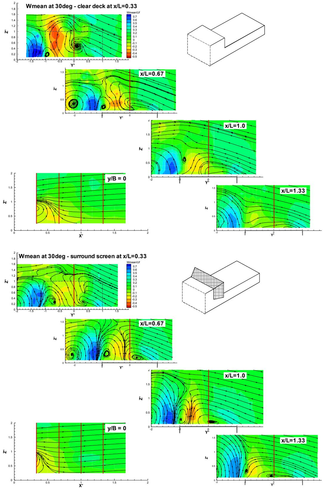
Figure 11. Effect of flow control on downwash distribution with 30° crosswind
