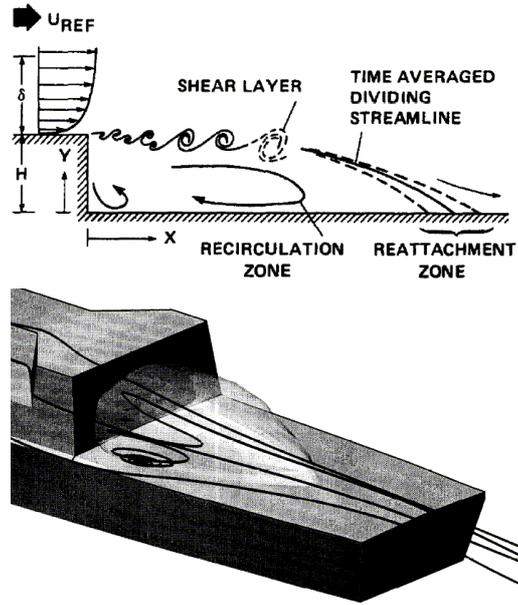
Figure 1. Flight deck recirculation zone [4,8]
