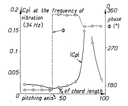
Fig. 10 – Fluctuating pressure distribution on the lower surface at  $i = 8^{\circ}$  and Mach 0.9.
