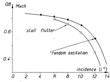
Fig. 11 – Comparison between the limiting conditions for stall flutter and for random excitation.
