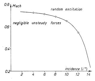
Fig. 7 – Limits of large random pressure fluctuations.
