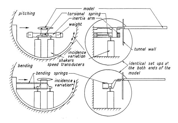
Fig. 2 - Test set-up.
