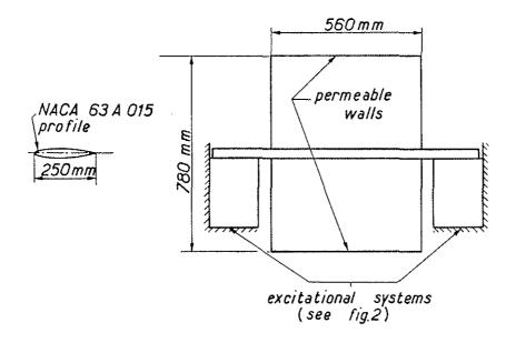
Fig. 1 - Wind tunnel and model.
