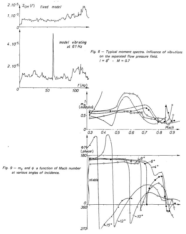
The phase reference chosen is such that the aerofoil is unstable when 180°  $\angle$   $\psi$   $\angle$  360°.
