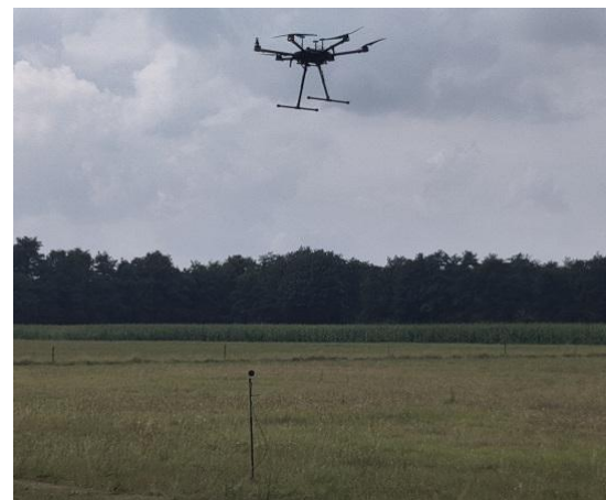
Figure 12: Picture of M600 drone, hovering above free-field microphone outside of DigiCity zone.
